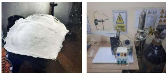
Figure 3: (a) The sample of PCL/Chitosan nanofiber (b) plasma jet set –up.
