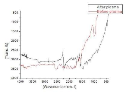
Figure 4: FTIR of the electrospun nanofiber PCL/Chitosan (before /after) plasma Jet at 0.4%
