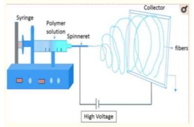
**Figure 1:** the electrospinning process
