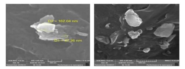
**Figure 5:** FESEM images of plasma treated electrospun nanofibers plasma jet of (0.05% and 0.4%) Cs.
