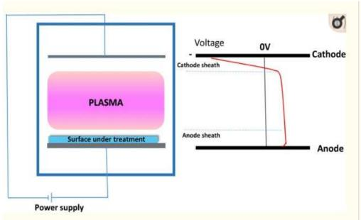
Figure 2: Plasma treatment on polymer surface [7].
