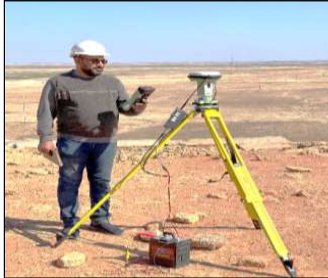
Figure 3: Observations methods static and (RTK) by GNSS receiver.
