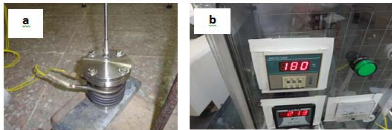
Figure 1- a-Hydrothermal reaction autoclave, b- An electric temperature regulating control board
