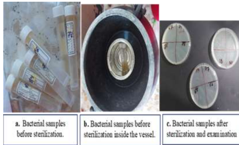
Figure 4: Photographs of bacteria samples prior to sterilization inside the solar autoclave and sterilization test results
