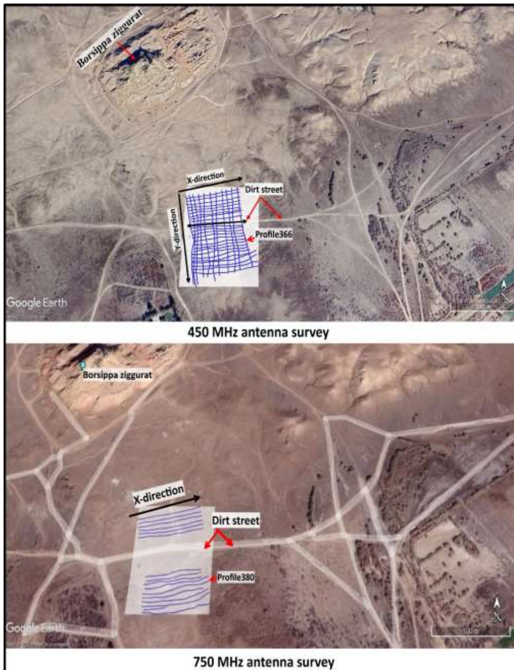
Figure 2: Google Earth Maps displays the locations of 450 MHz antenna profiles and 750 MHz antenna profiles.
