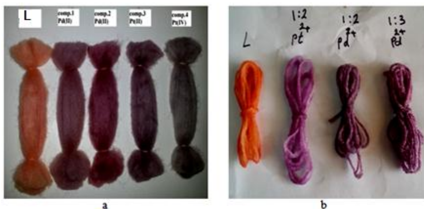
Figure 15- Dyeing of a- 100% wool and b- 100% acrylic by the ligand and its complexes
