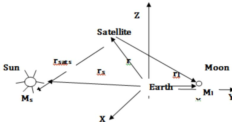
**Figure 1-** Vectors and gravitational force of the Sun and the Moon on the Earth satellite
