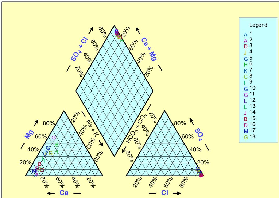
Figure 5- Piper diagram illustrates the groundwater chemistry type.
