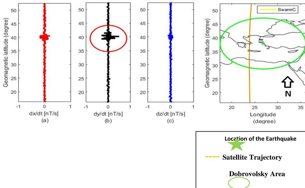
**Figure 3:** The AMSW algorithm detects anomalous events at 01:30 UTC and 03:35 LT on October 23, 2020, at SW- C, seven days before October 30, 2020,  $M = 7.0$ . Dobrovolsky's region is the green circle surrounding the epicenter, and the red line is the orbit of the Swarm satellite.
