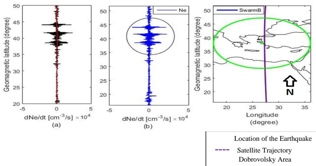
**Figure 4:** The AMSW algorithm detects anomalous events at 01:03 UTC and 02:30 LT on May 26, 2020, at SW- B, 155 days before Oct 30, 2020, with  $M = 7.0$ . Dobrovolsky's region is the green circle surrounding the epicenter, and the redline is the orbit of the Swarm satellite.
