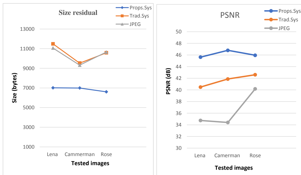
Figure 4: The comparison performance between the standard JPEG, the proposed system, and the traditional system [15] in terms of a) Size system and b) PSNR for tested images.
