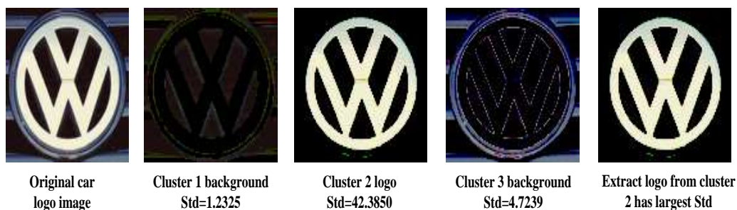
Figure 5: The result of standard deviation and extract logo from larger standard deviation
