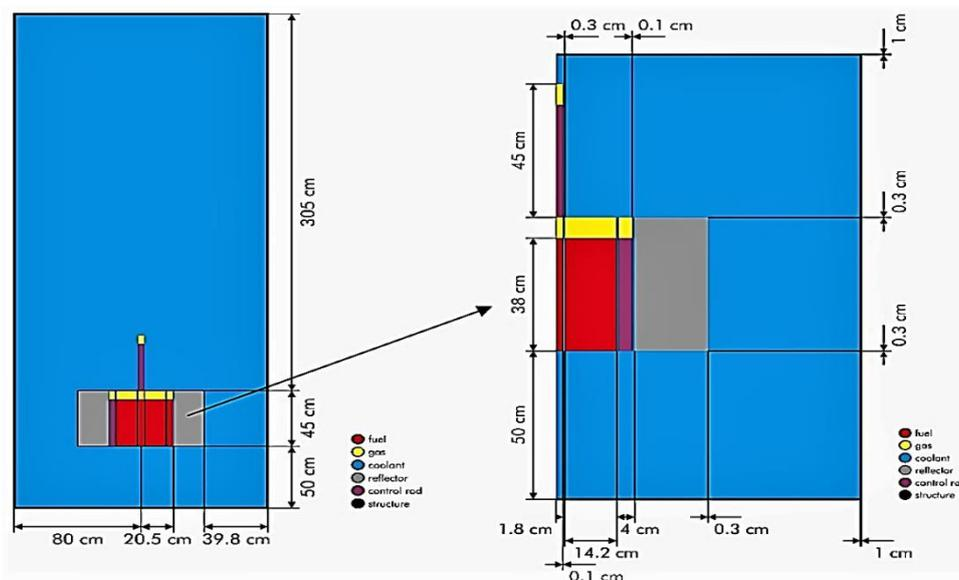
**Figure 2:** ADS-SAMOP reactor technical configurations: reactor core and water coolant tank
