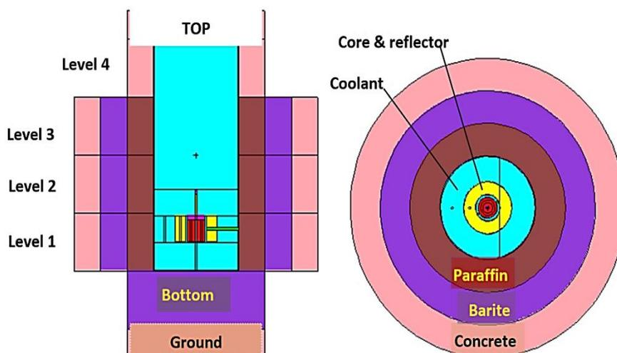
**Figure 3:** ADS-SAMOP reactor configuration using 50 cm of paraffin, 50 cm barite and 50 cm ordinary concrete as radial shielding
