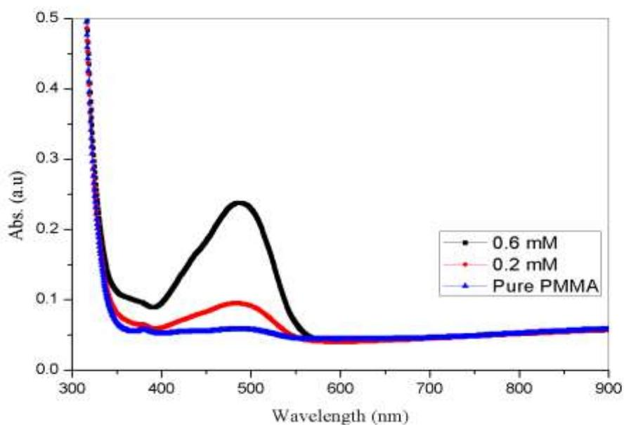
**Figure 2-**Absorption spectrum of pure and doped PMMA by BCG dye.
