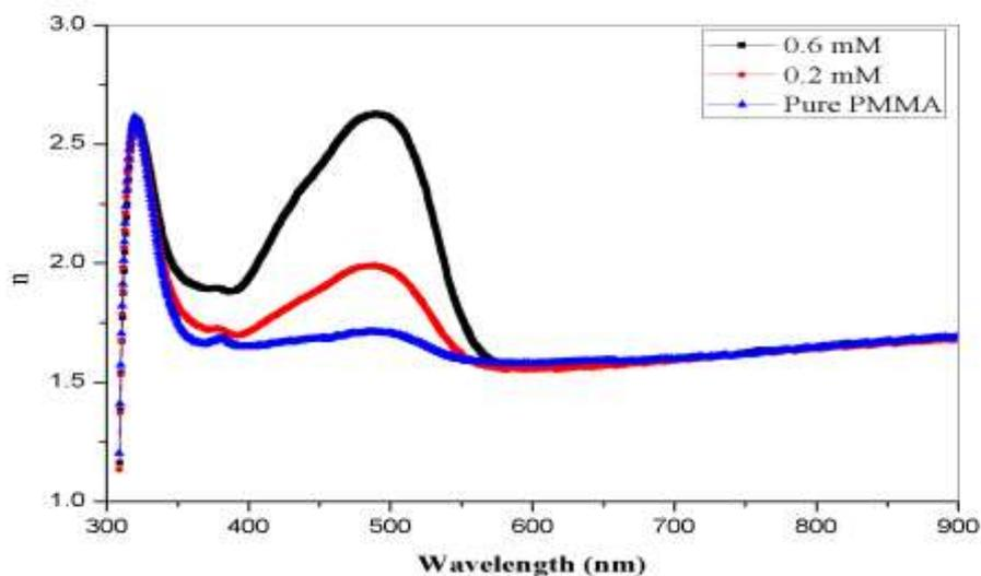
**Figure 5-**Refractive index of pure and doped PMMA by BCG dye.
