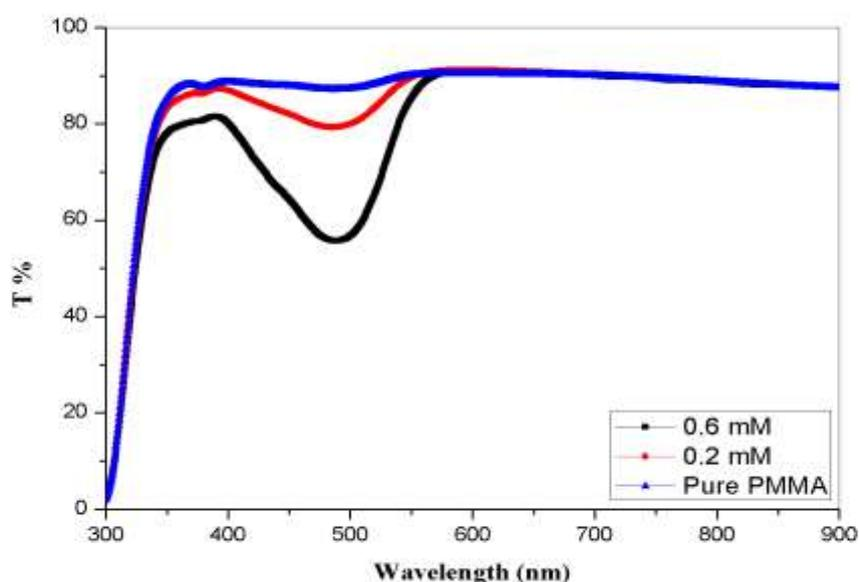
**Figure 3-**Transmittance spectrum of pure and doped PMMA by BCG dye.
