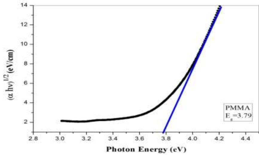
Figure 9 (A)-Indirect energy gap of pure PMMA polymer.
