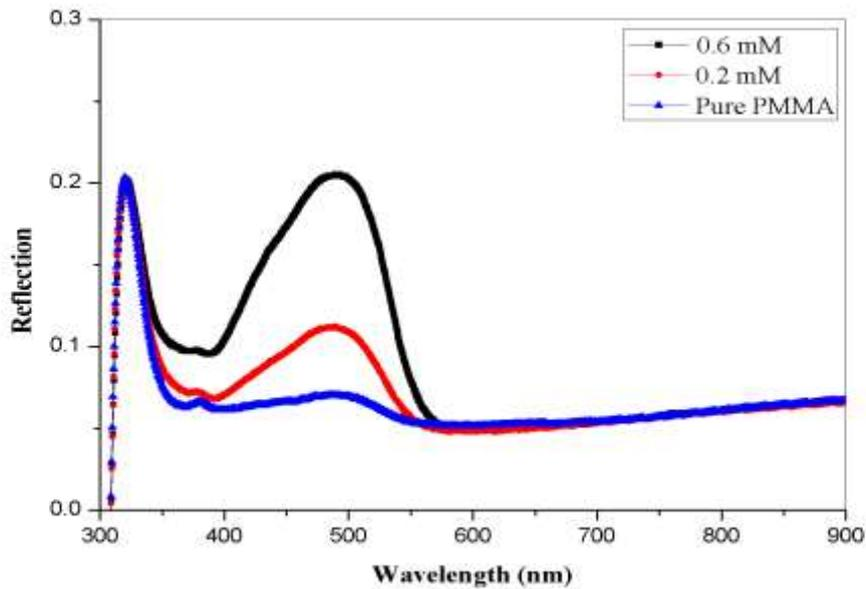
**Figure 4-**Reflection spectrum of pure and doped PMMA by BCG dye.
