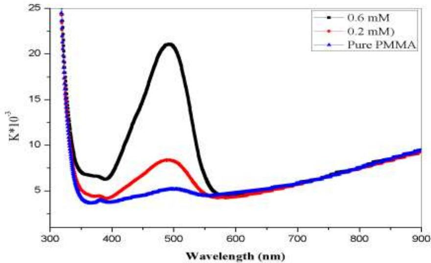
**Figure 6-**Extinction coefficient of pure and doped PMMA by BCG dye.
