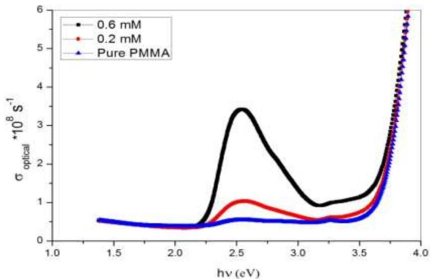
**Figure 7-**The optical conductivity of pure and doped PMMA by BCG dye.
