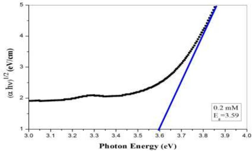
Figure 9(B)-Indirect energy gap of doped PMMA polymer at 0.2 m mol/L.
