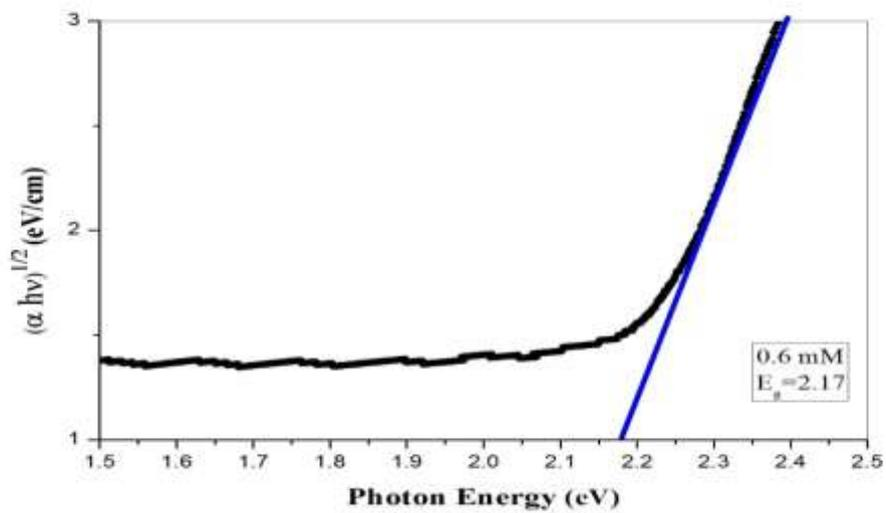
Figure 9(C)-Indirect energy gap of doped PMMA polymer at 0.6 m mol/L.
