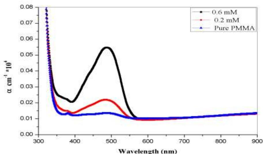
**Figure 8-**Absorption coefficient of pure and doped PMMA by BCG dye.
