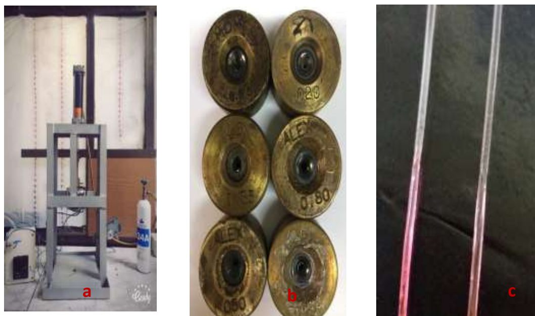
Figure 1- contracted system for withdrawing fiber, a: the core system, b specified diameter discs: the pulling fiber with doping clad
