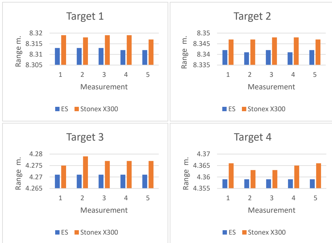
Figure 3: Compared with reference target measurements, the mean range errors of Stonex X300 were delivered from calibration targets (set 1).
