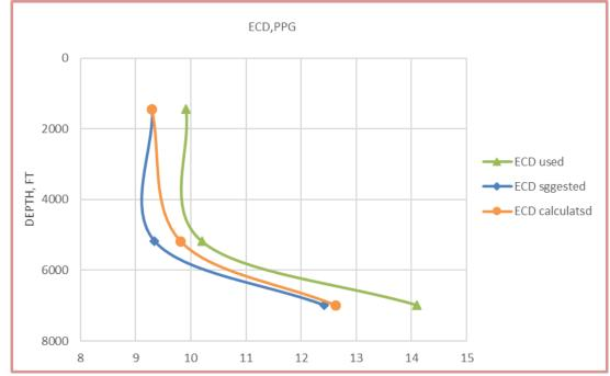
Figure 4- Comparison between used ECD, calculated ECD and suggested ECD
