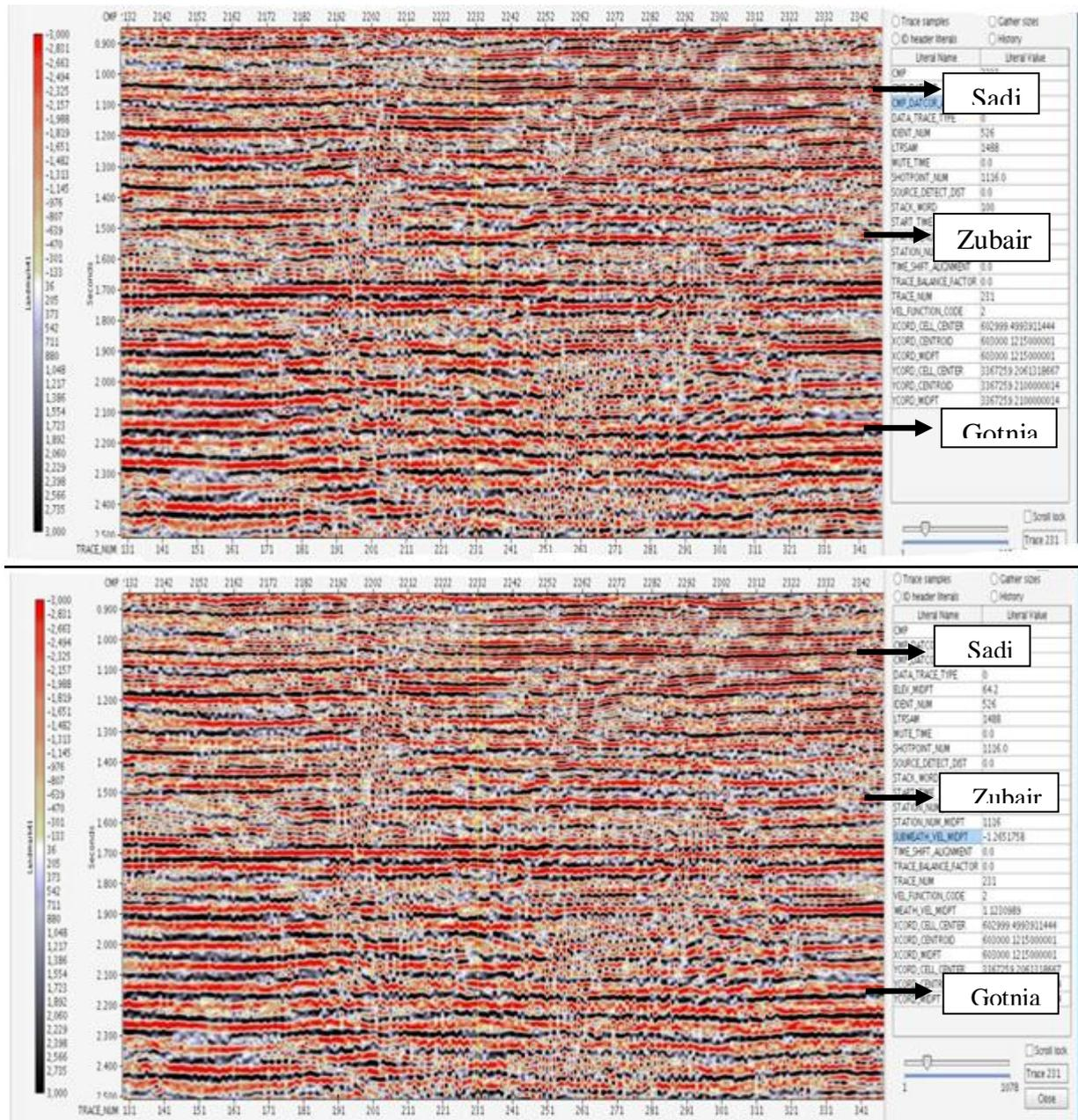
**Figure 11-** Final stacked sections: (top) before applying a residual static correction; (bottom) after applying a residual using elevation static for the line (2WL2).
