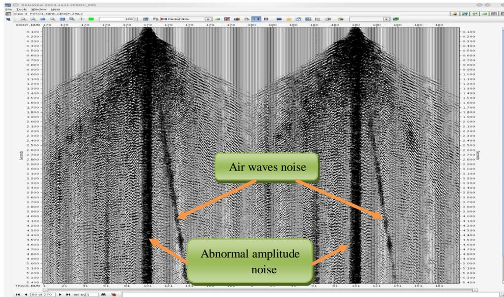
Figure 6- Types of noise that appeared in (2WL2) records which are removed from the seismic signal
