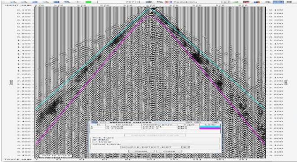
**Figure 8-** One pannal (10- 20 Hz) of band pass filter for (2WL4) records to show head waves frequency and velocity.
