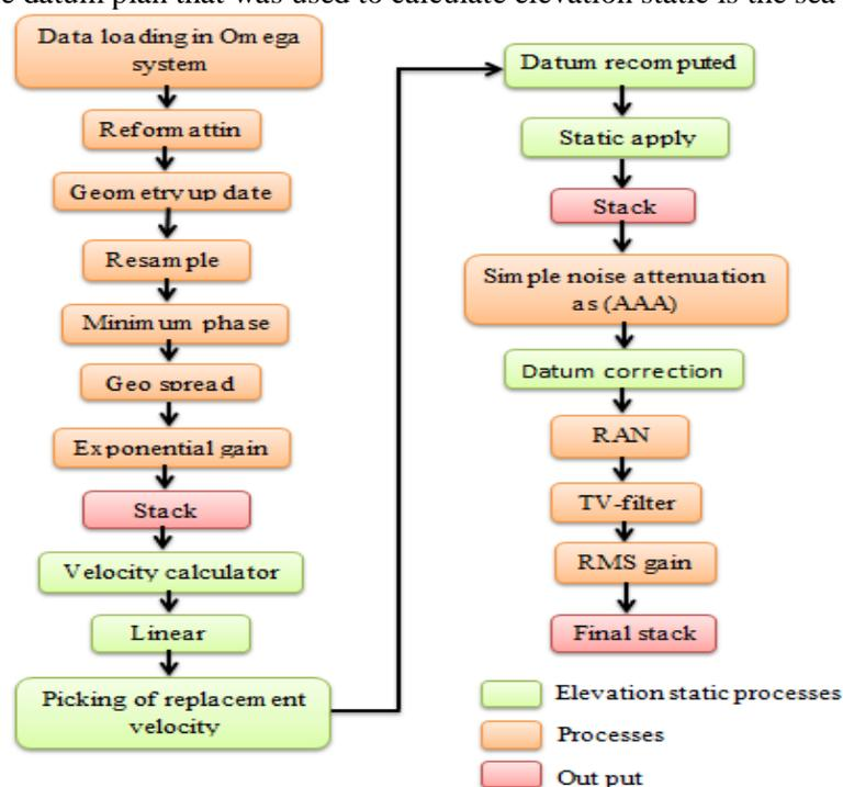
**Figure 3-** A Flow chart shows steps that are used for the calculation of elevation static correction to get the final stack.
