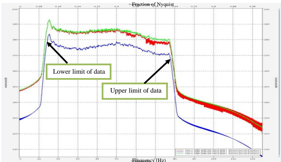
Figure 7- Spectral analysis of the test shots to know the limitations of signal and noise frequencies, the line blue is data field, the line green after gain apply and the line red represented data after noise attenuation process apply.
