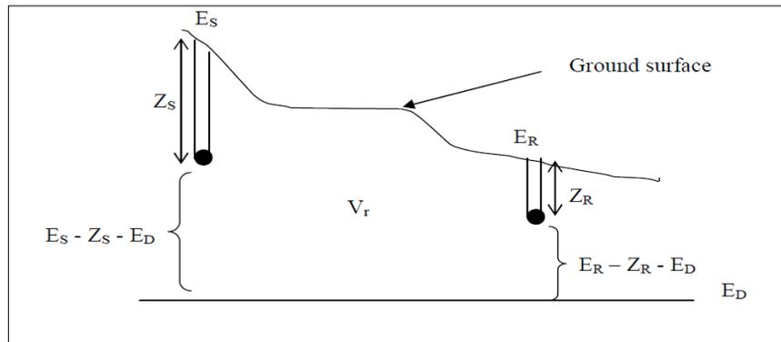
**Figure 2-** Simple model illustrating the symbols used in static correction computation.
