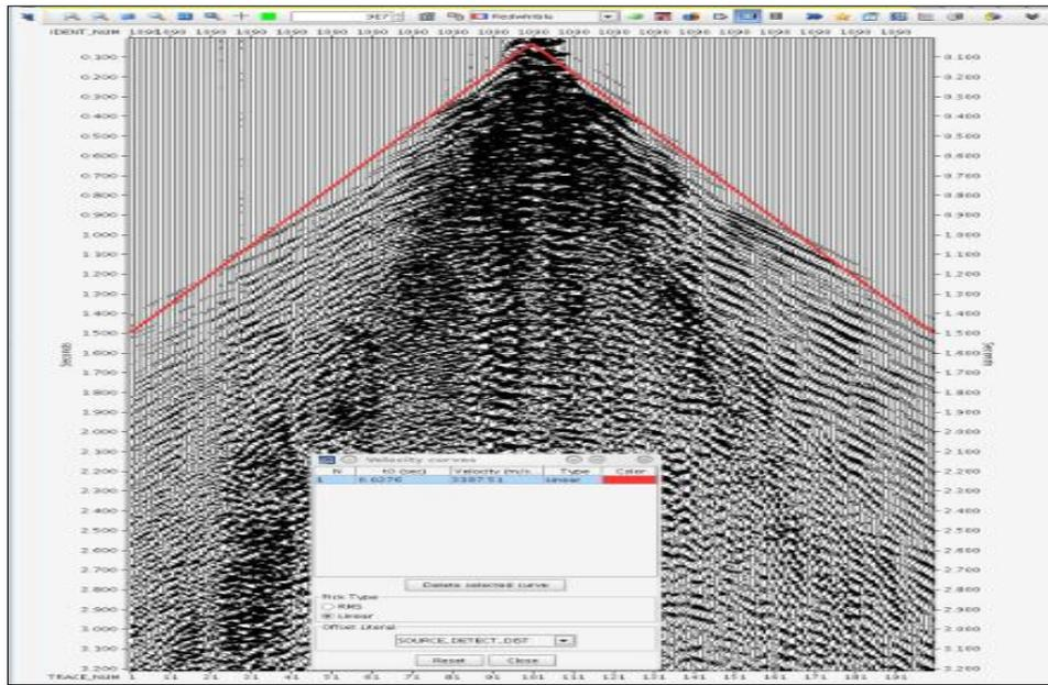
**Figure 4-** Picking of replacement velocity.
