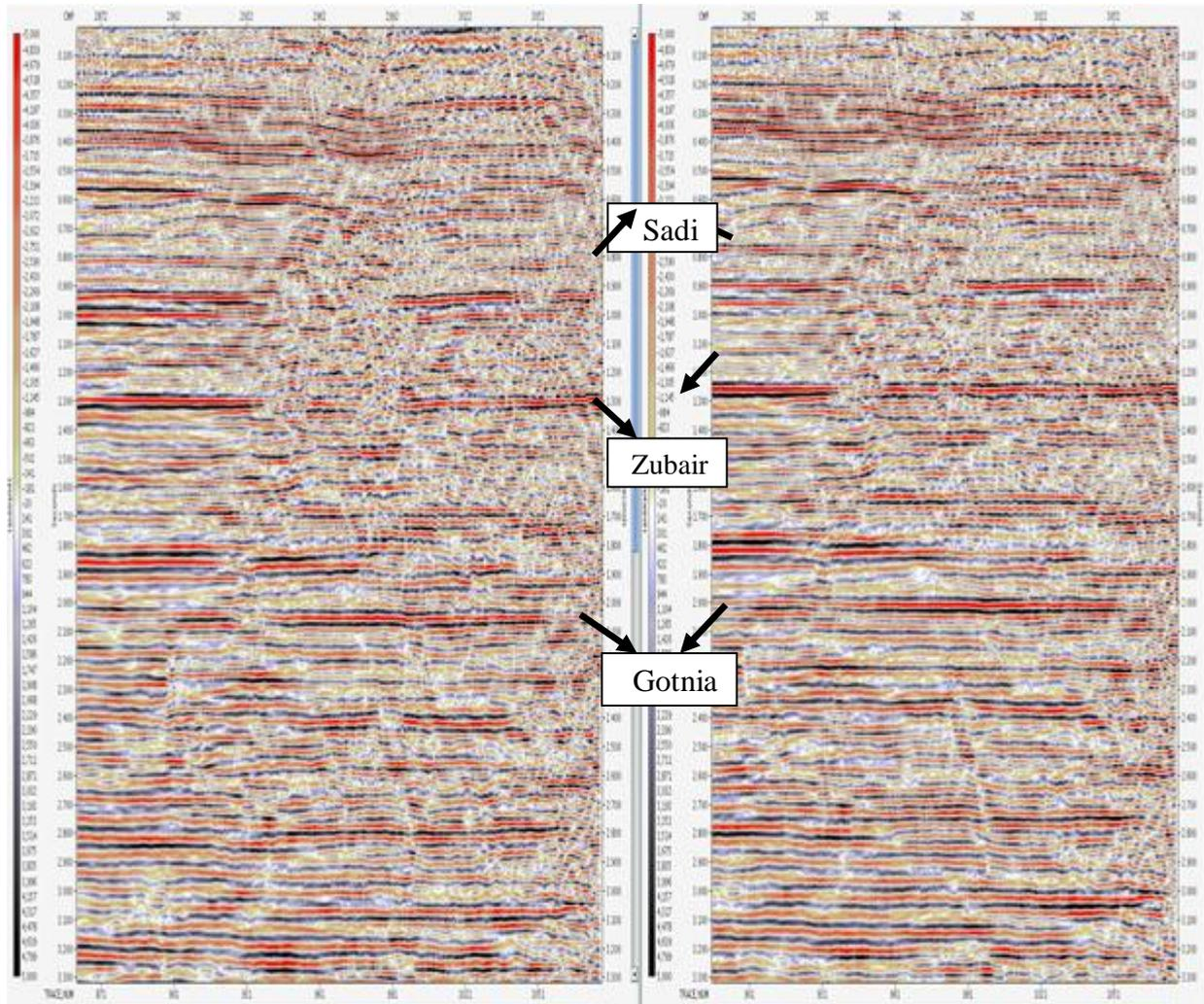
**Figure 10-** Final Stacked sections for (2WL2): (left) before applying elevation static correction; (right) after applying elevation static correction.
