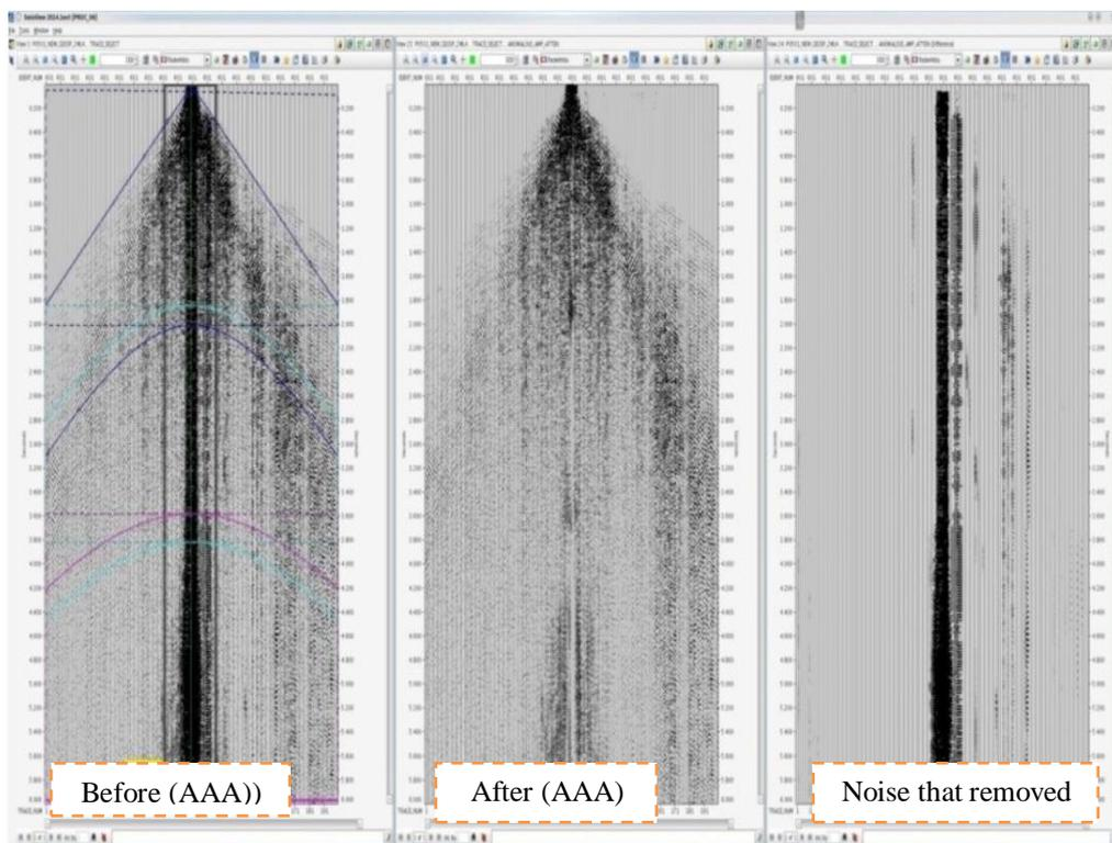
**Figure 9-**Using of (AAA) process on a given field record (2WL2).
