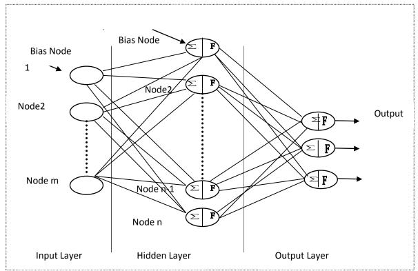
Figure 4- BPNN Structure of VDS
