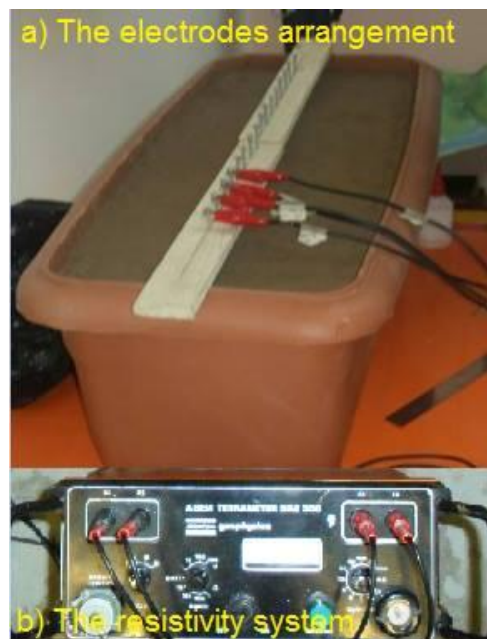
Figure 2- The acquisition system (a- side view to electrode arrangement and container, b- top view to instrument used SAS300)
