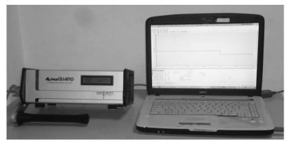
Figure 2- ALPHA GUARD radon monitor used in current study
