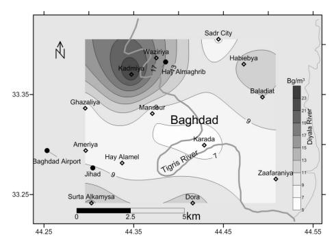
Figure 6- contour map shows the distribution of radon in city of Baghdad. Contour interval is 2 Bq/m<sup>3</sup>.
