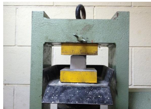
Figure 9- Rock sample during test.
