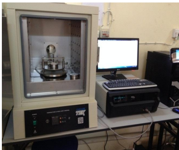
Figure 12- Samples in the hot disk machine
