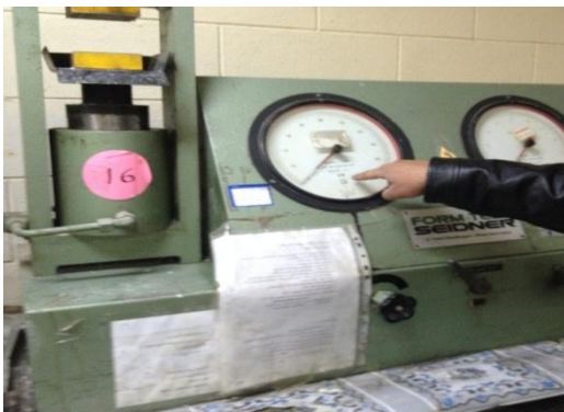
Figure 8- Compressive strength test machine.
