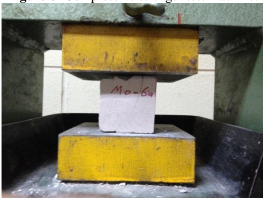
Figure 10- Failure of rock sample.
