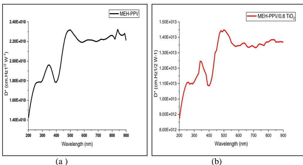
Figure 8-The Detectivity of a) MEH-PPV, b) MEH-PPV/0.8 (Rutile) TiO<sub>2</sub> nanocomposite
