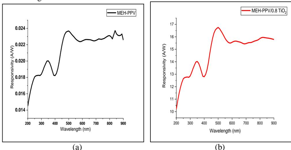
**Figure 5-**The Responsivity of a) MEH-PPV, b) MEH-PPV/0.8 (Rutile)  $TiO_2$  nanocomposite.
