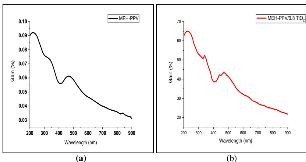
**Figure 6-**The Gain of a) MEH-PPV, b) MEH-PPV/0.8 (Rutile)  $TiO_2$  nanocomposite.
