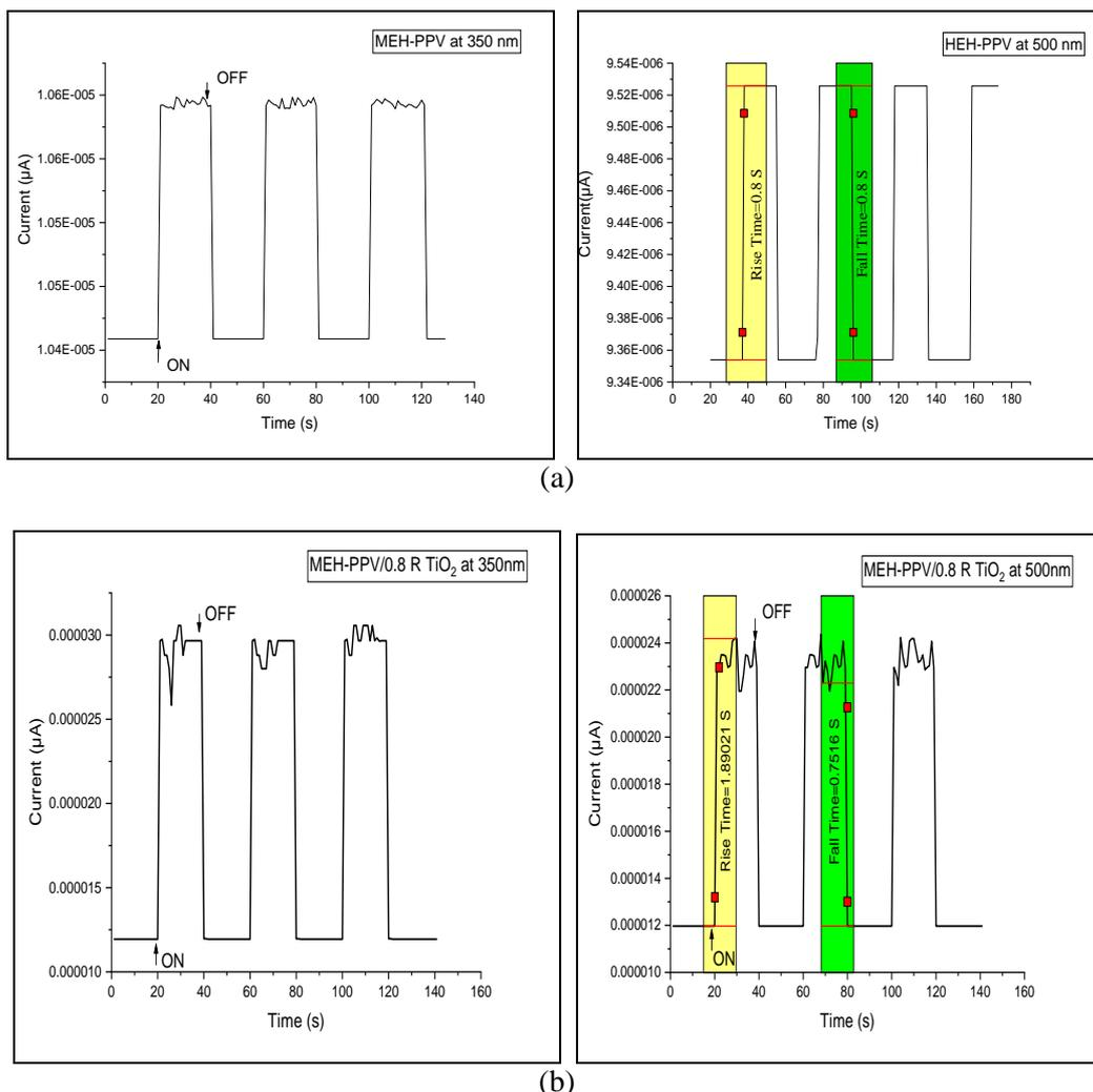
**Figure 9**-the time-dependent photocurrent of the MEH-PPV/(Rutile)TiO<sub>2</sub> in the excitation wavelength (350 and 500) nm (a ) MEH-PPV, (d) MEH-PPV/0.8 Rutile TiO<sub>2</sub>
