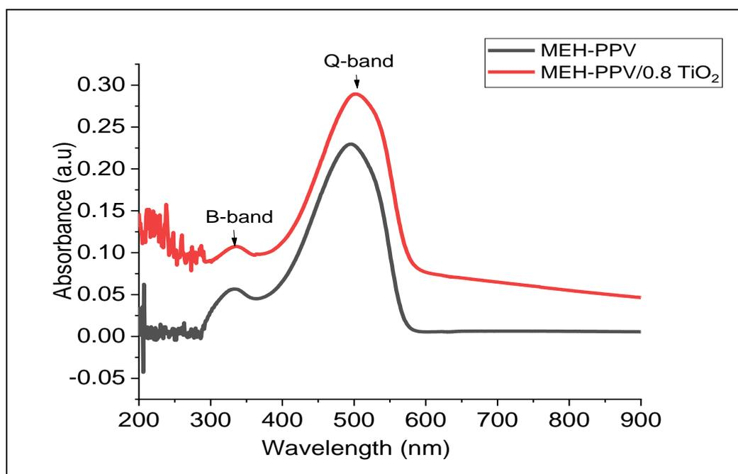
**Figure 2-**The absorption spectra of MEH-PPV and (MEH-PPV/0.8 Rutile  $\text{TiO}_2$ ) Nanocomposite thin films.
