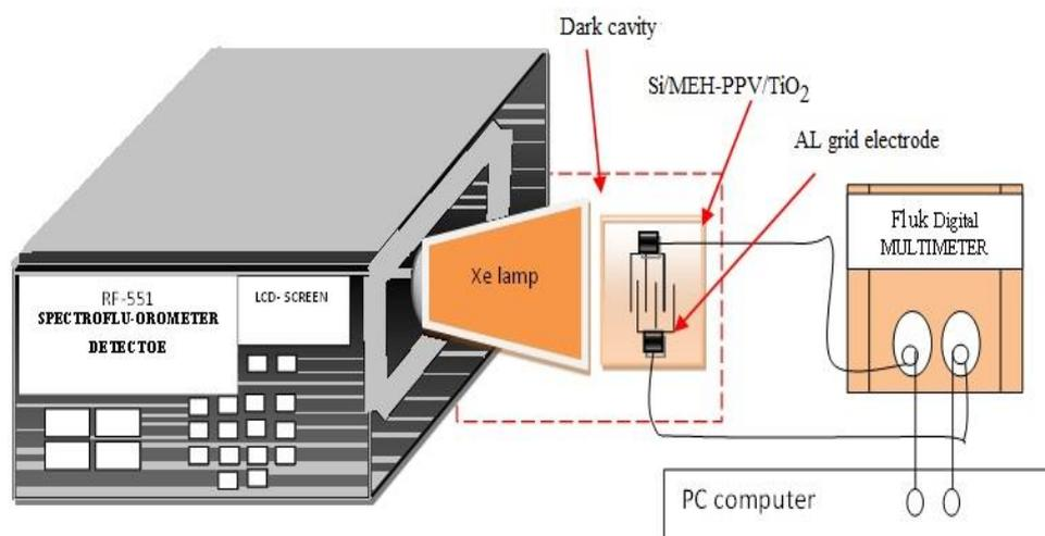
**Figure 1-A** schematic of the photoconductive sample
