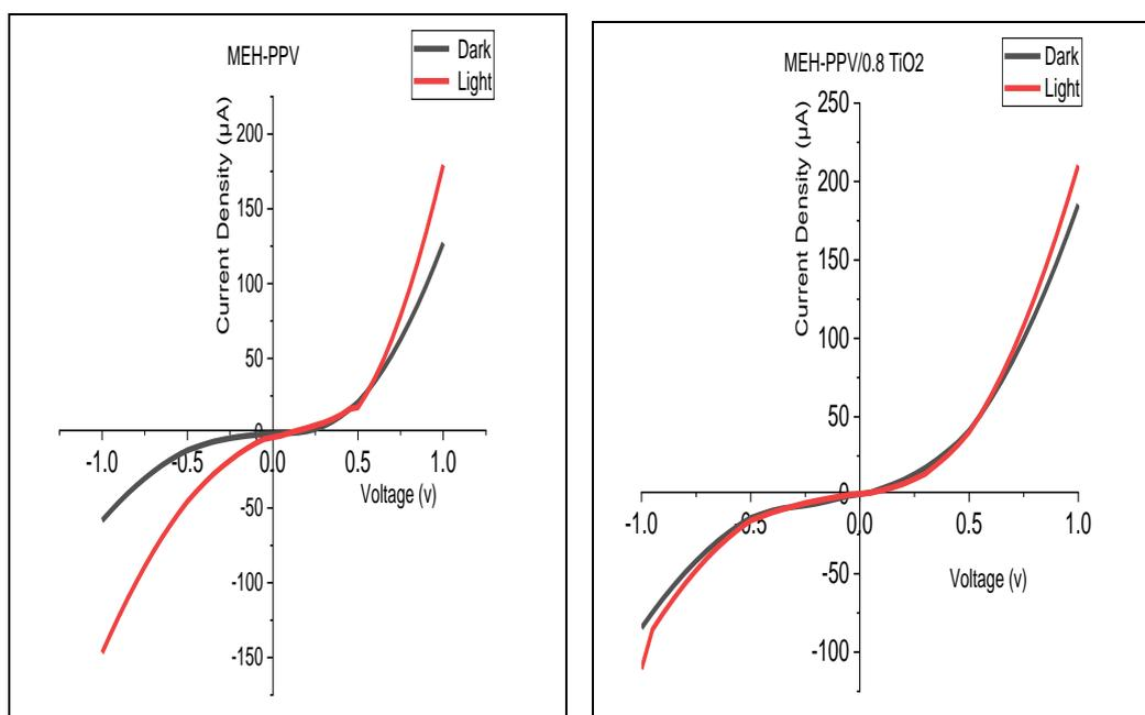
**Figure 3-**Current – Voltage comparison between Dark and Light ( $104.98 \text{ mW/cm}^2$ ) of a) MEH-PPV and b)MEH-PPV/0.8  $\text{TiO}_2$  thin films
