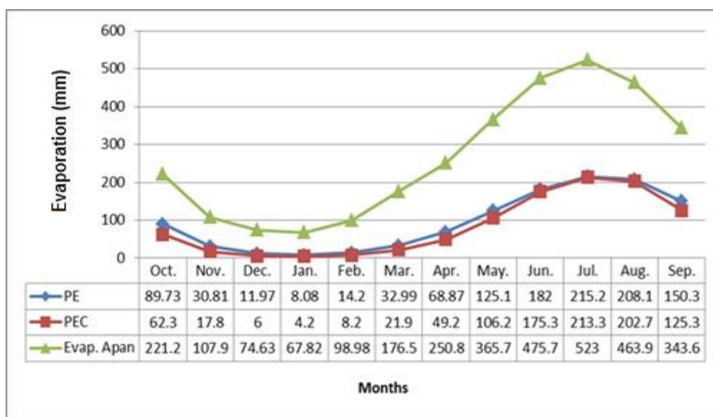
Figure 6: Evaporation, potential evapotranspiration (PE) and corrected potential evapotranspiration (PEc) correlation line graph at Baghdad Airport and Al-Ramadi Meteorological Station (1989-2020).
