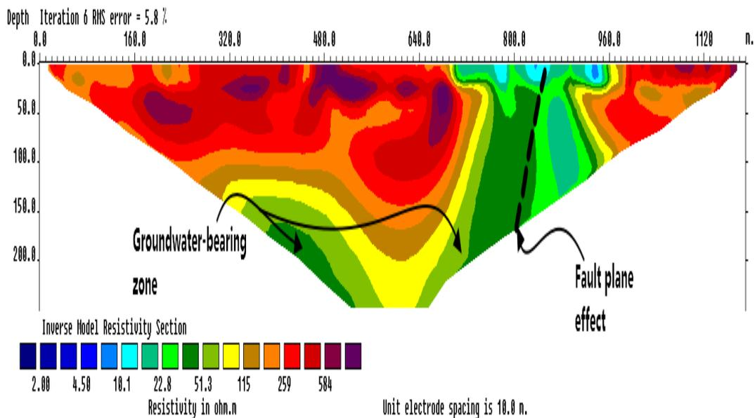
**Figure 7-** Inverse model of the survey point 2-D SH 4.
