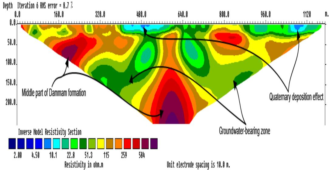
Figure 9- Inverse model of the survey point 2-D SH 6.
