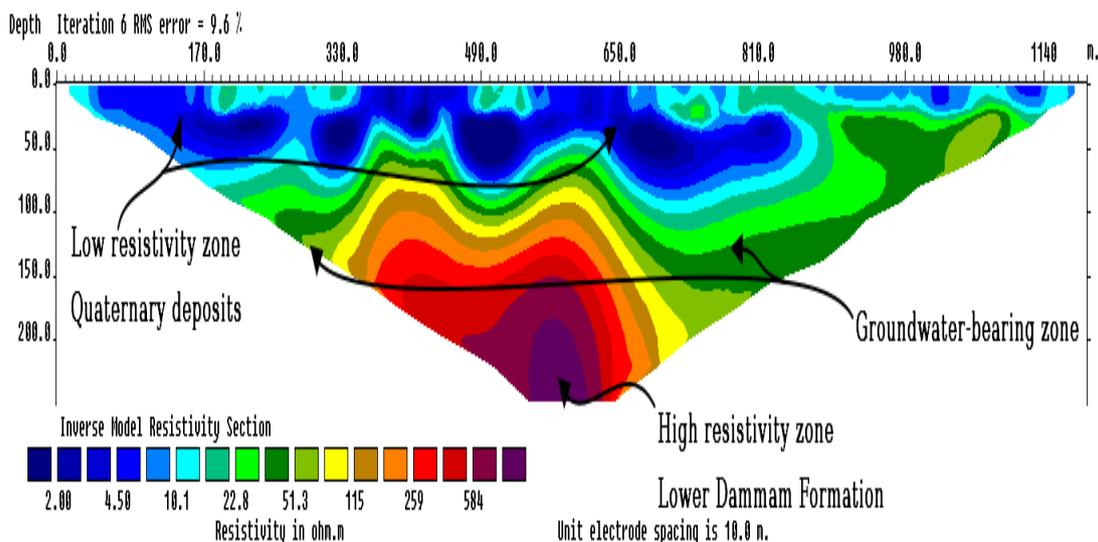
Figure 5- an Inverse model of the survey point 2-D SH 2.
