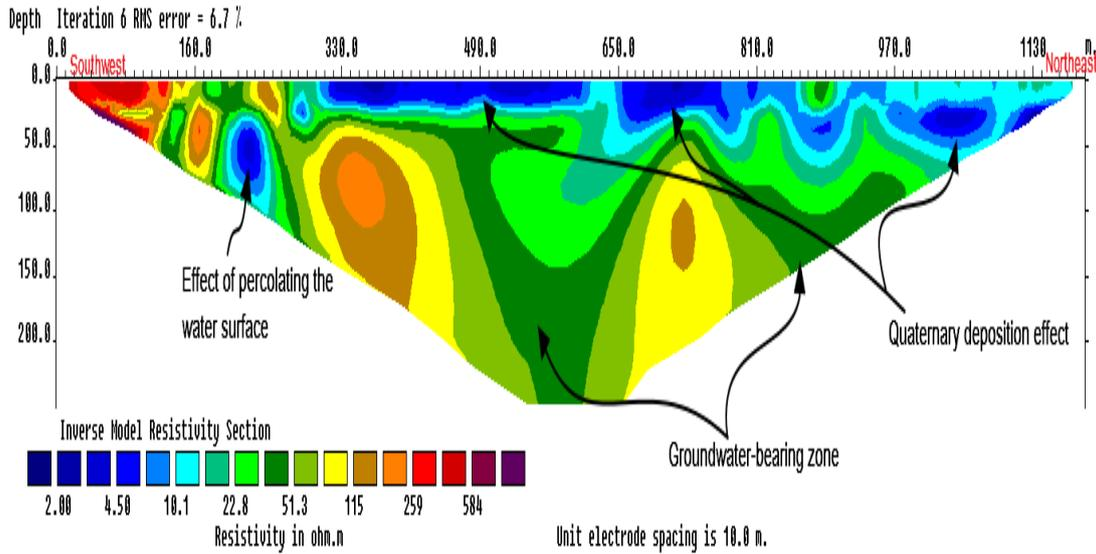
**Figure 11-** the Inverse model of the survey point 2-D SH 8.
