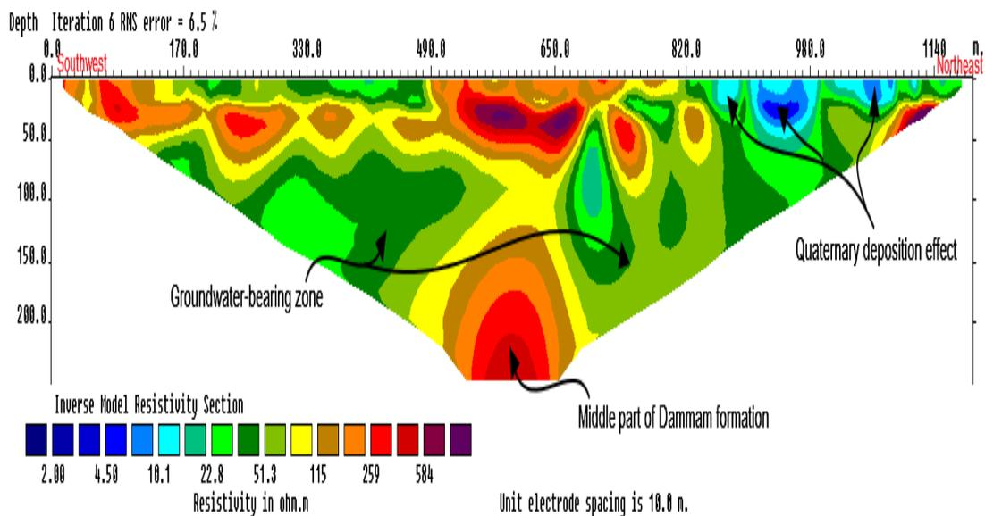
**Figure 8-** Inverse model of the survey point 2-D SH 5.
