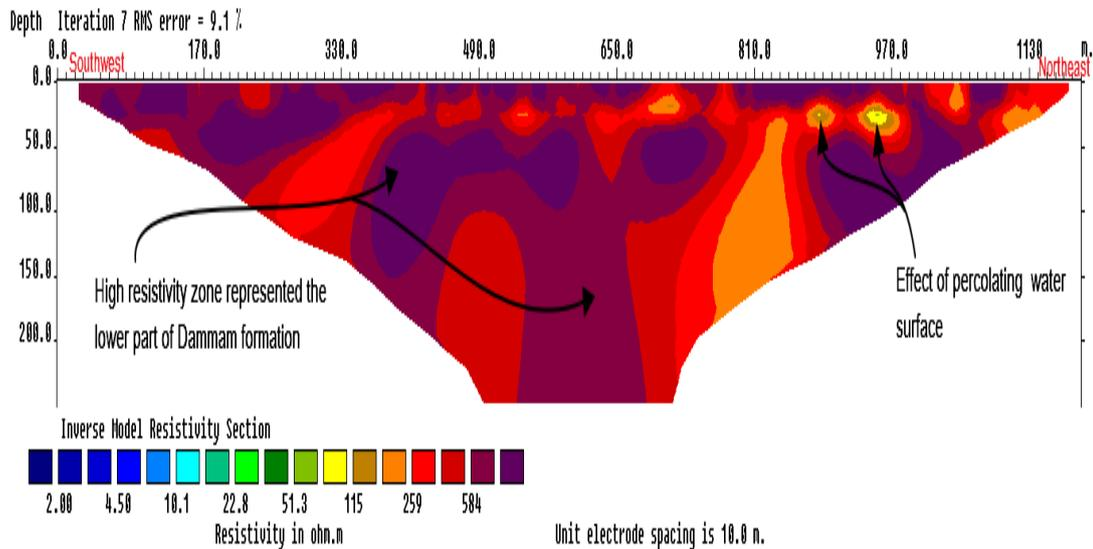
**Figure 13-** the Inverse model of the survey point 2-D SH 10.
