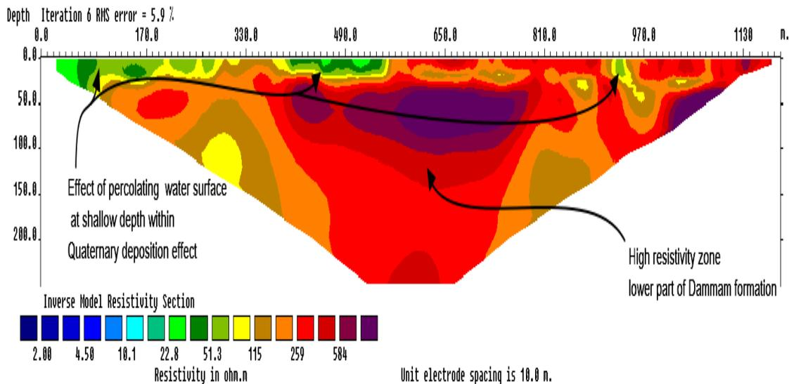
**Figure 12-** Inverse model of the survey point 2-D SH 9.
