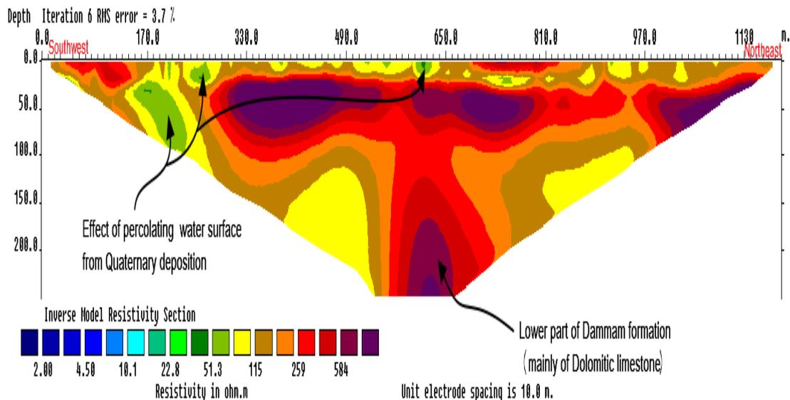
Figure 10- the Inverse model of the survey point 2-D SH 7.
