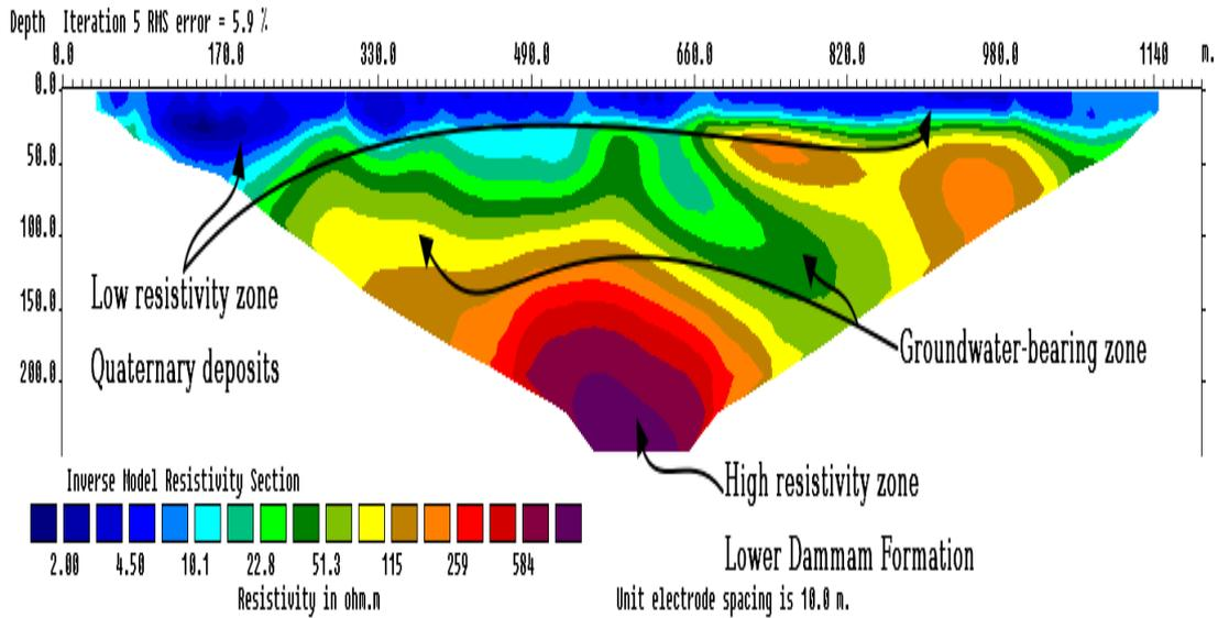
Figure 4- the Inverse model of the survey point 2-D SH 1.
