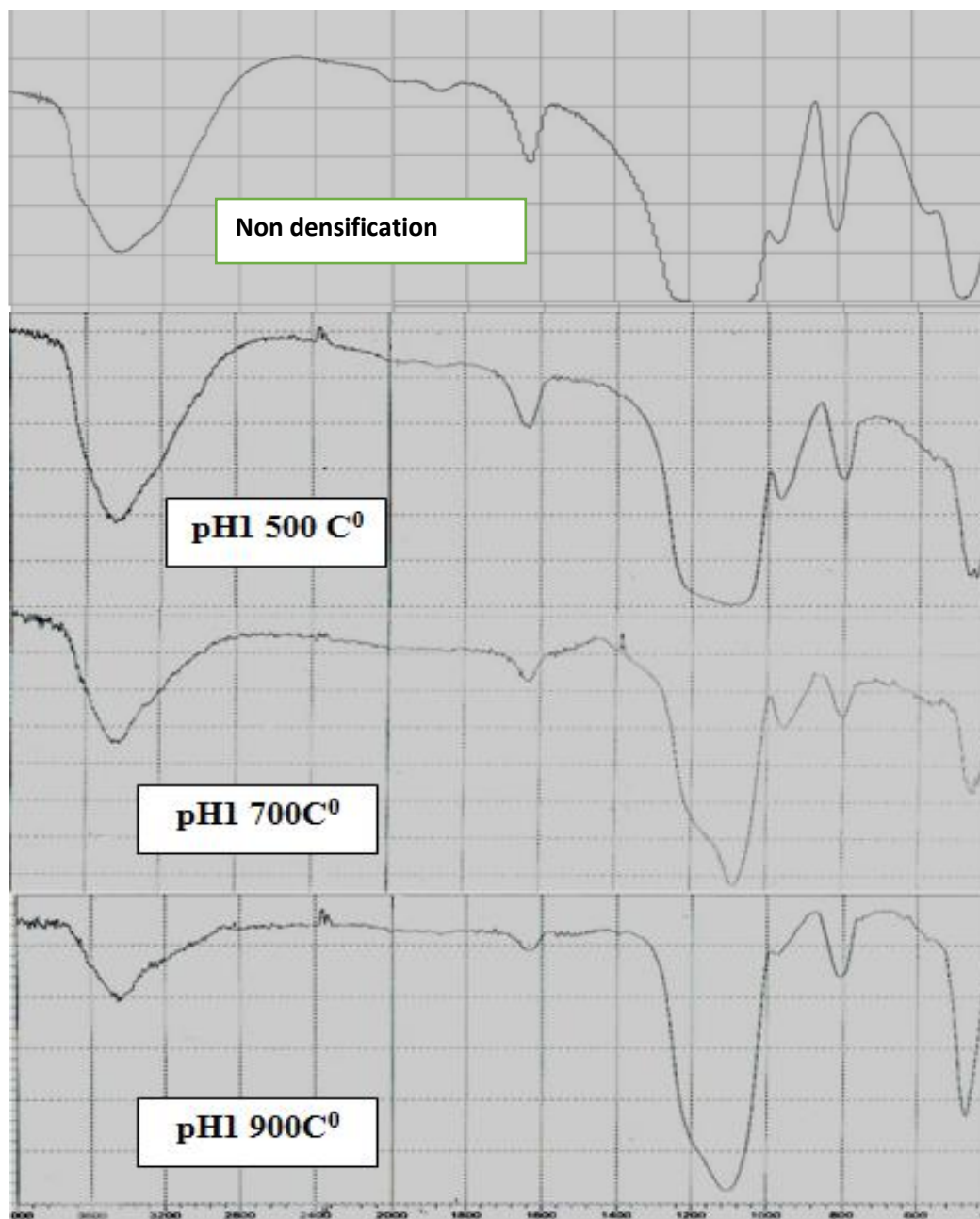
Figure 5- FTIR transmission spectra for aerogel sample pH=1 at three different annealing temperatures 500 °C, 700 °C and 900 °C.
