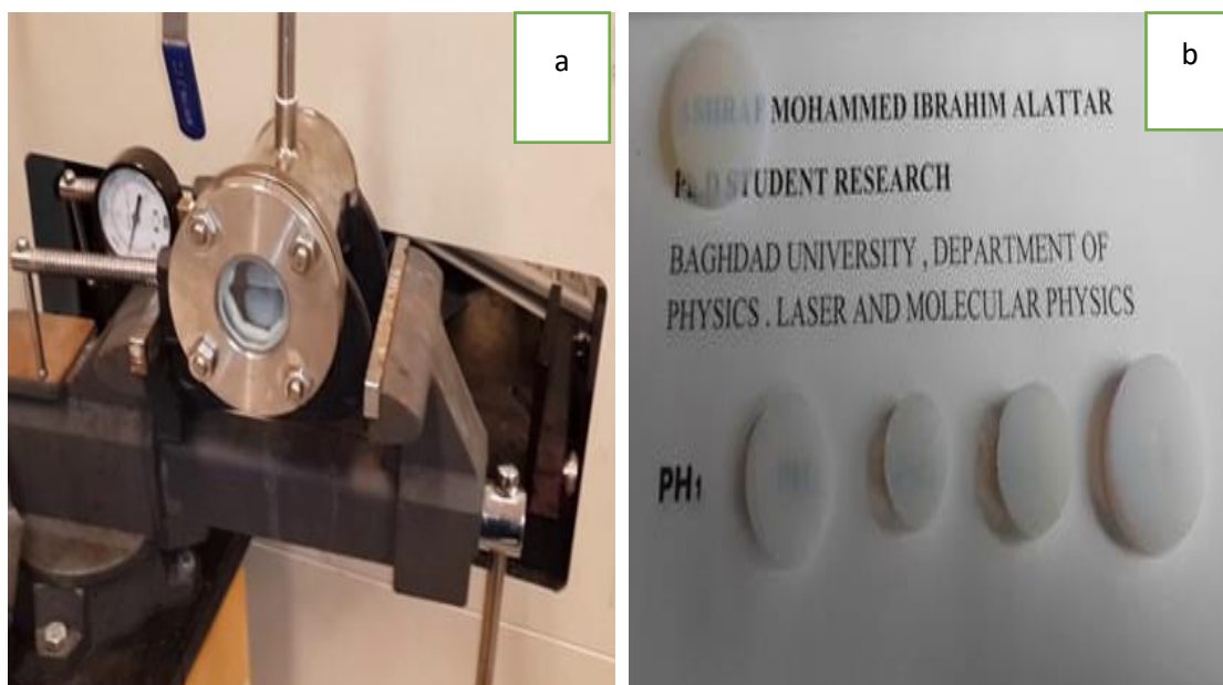
Figure 1 -Camera image forPhotos of (a) Implemented autoclave, (b) some aerogel samples with their preparation pH1 value.
