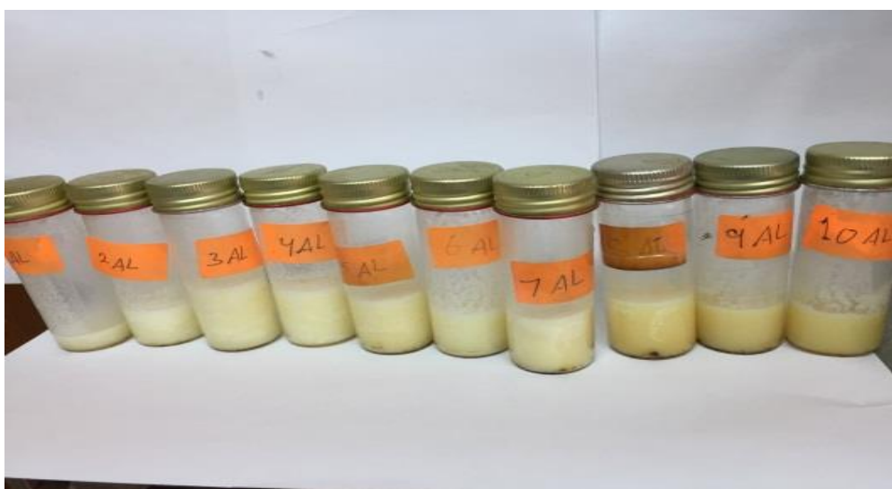
Figure 3- photographic picture of vegetable oil heated and stored six months in Aluminum pan.
