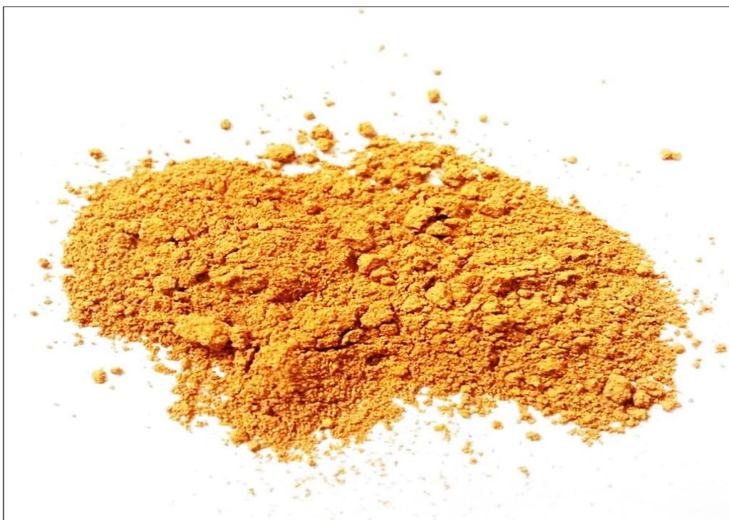
**Figure 1-** acidic activated bentonite.
