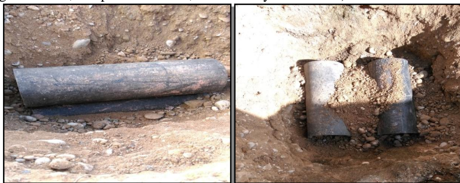
Figure 1 – Lined Horizontal and vertical iron pipes inside the dry mixture clastic deposit model.
