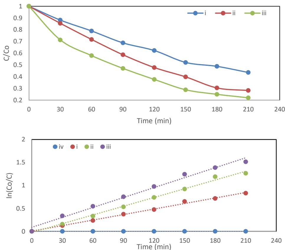
**Figure 9-** (a) Typical variation in the normalized residual MB dye concentration as a function of UV-exposure time, obtained for the mixed-phase nanocrystalline  $\text{TiO}_2$  processed via DC Magnetron Sputtering Technique with a rutile content of (i) 38 wt.%,(ii) 43 wt.%, and (iii) 53 wt.%, (iv) absence of nanocrystalline  $\text{TiO}_2$  (b) Typical plots, obtained using part a
