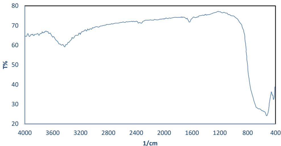
**Figure 4-**FT-IR spectra of TiO<sub>2</sub> sample with relative amounts of rutile of 43%.
