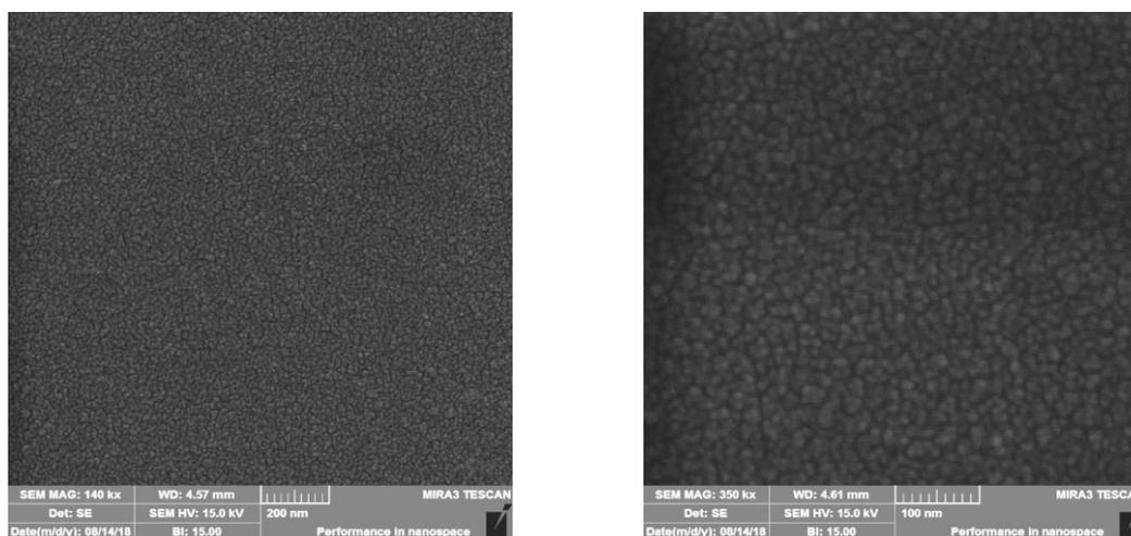
**Figure 5-**SEM image of TiO<sub>2</sub> sample with relative amounts of rutile of 43%.
