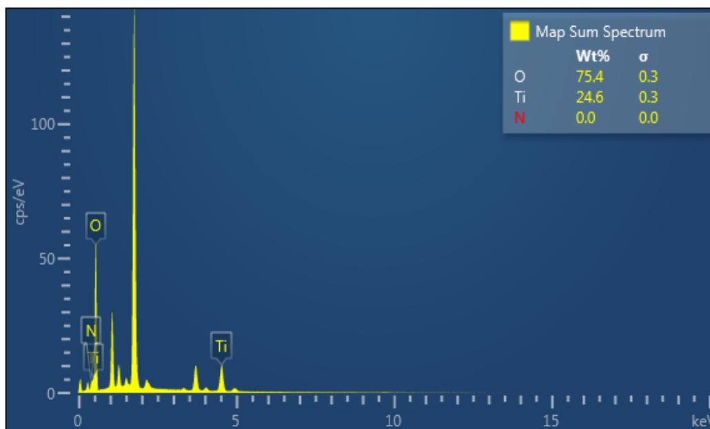
Figure 6-EDX image of TiO<sub>2</sub> sample with relative amounts of rutile of 43%.
