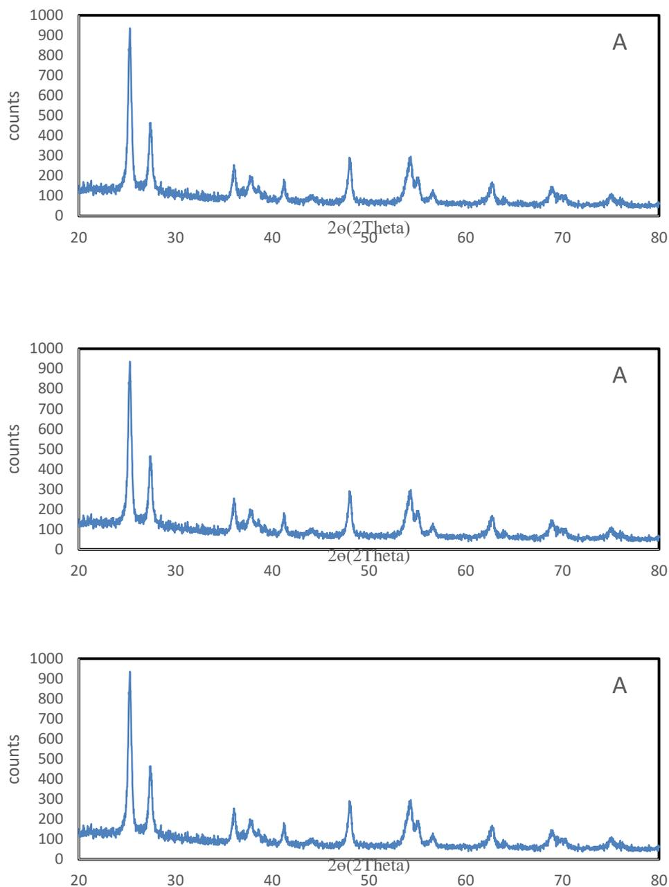
**Figure 3**-Broad-scan XRD spectra obtained for mixed-phase nanocrystalline  $\text{TiO}_2$  processed via D.C. CFRMSS at deposition time (a) 3.5 hour, (b) 4 hour, and (c) 4.5 hour .A and R represent diffraction peaks corresponding to anatase- $\text{TiO}_2$  and rutile- $\text{TiO}_2$ , respectively.
