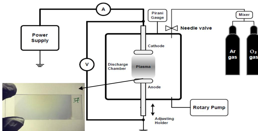
**Figure 2**-Schematic diagram of the home made CFDCMS configuration
