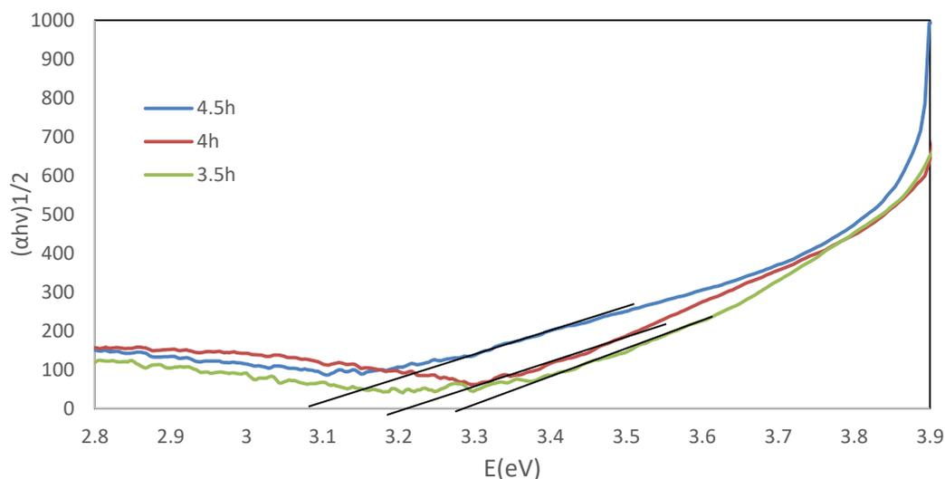
**Figure 8**-Energy band gap determination of  $\text{TiO}_2$  samples at deposition time 3.5 hour (rutile content 38 wt.%), 4 hours (rutile content 43 wt.%) and 4.5 hours (rutile content 53 wt.%).
