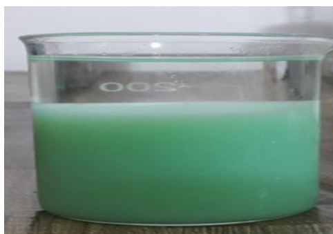
Figure 1 -Green gel of NiO nanoparticles
