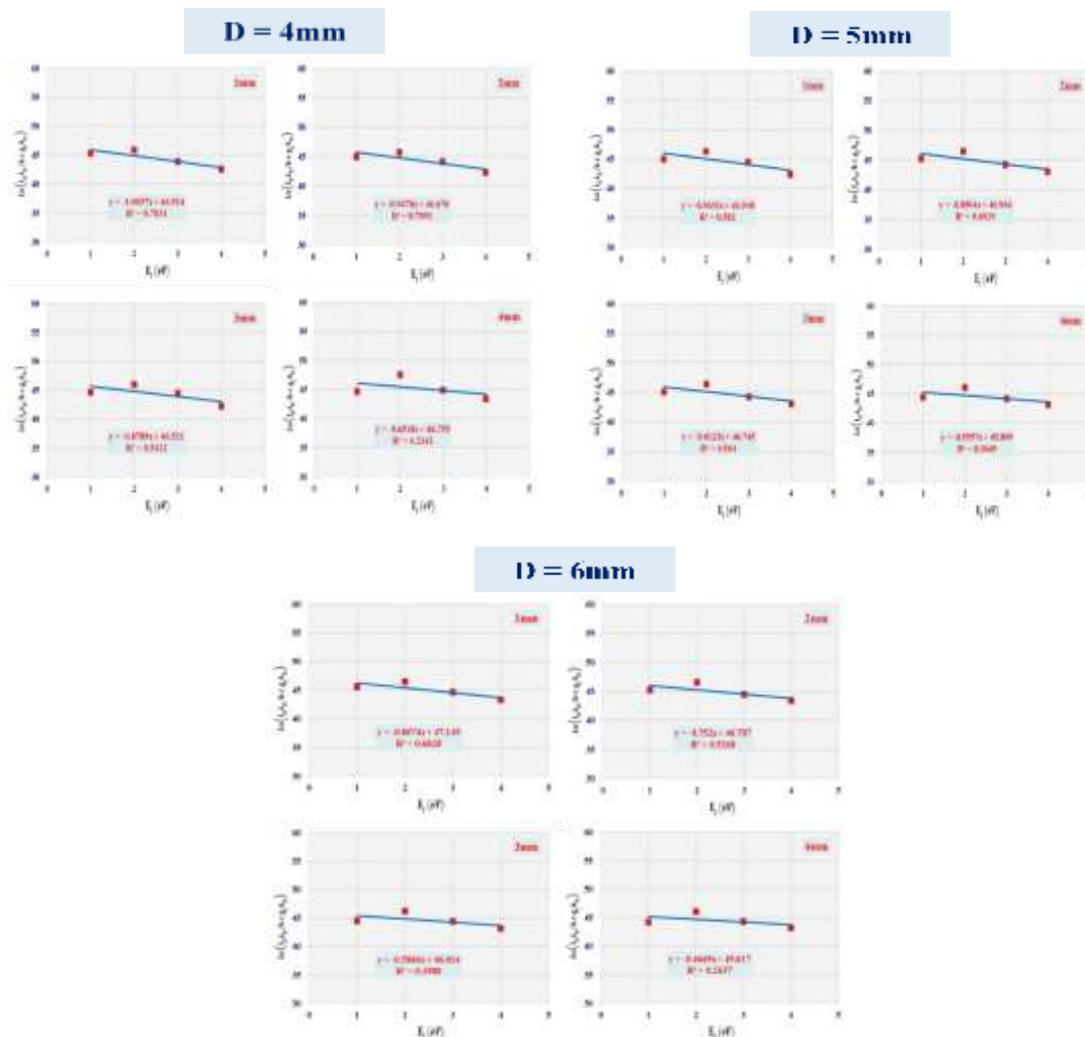
**Figure 4:** Boltzmann plots for N I peaks at varying gap distances (1, 2, 3, and 4mm) with different cathode diameters (4, 5, and 6mm).
