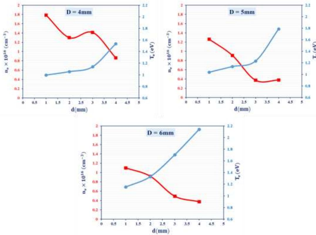
**Figure 5:** The Variation of  $n_e$  and  $T_e$  of the plasma emitted from rod-plate electrodes as a function of the distance between the electrodes for different cathode diameters.
