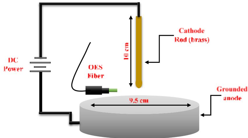
**Figure 1:** A schematic diagram of the rod-plate cathode DC discharge setup.
