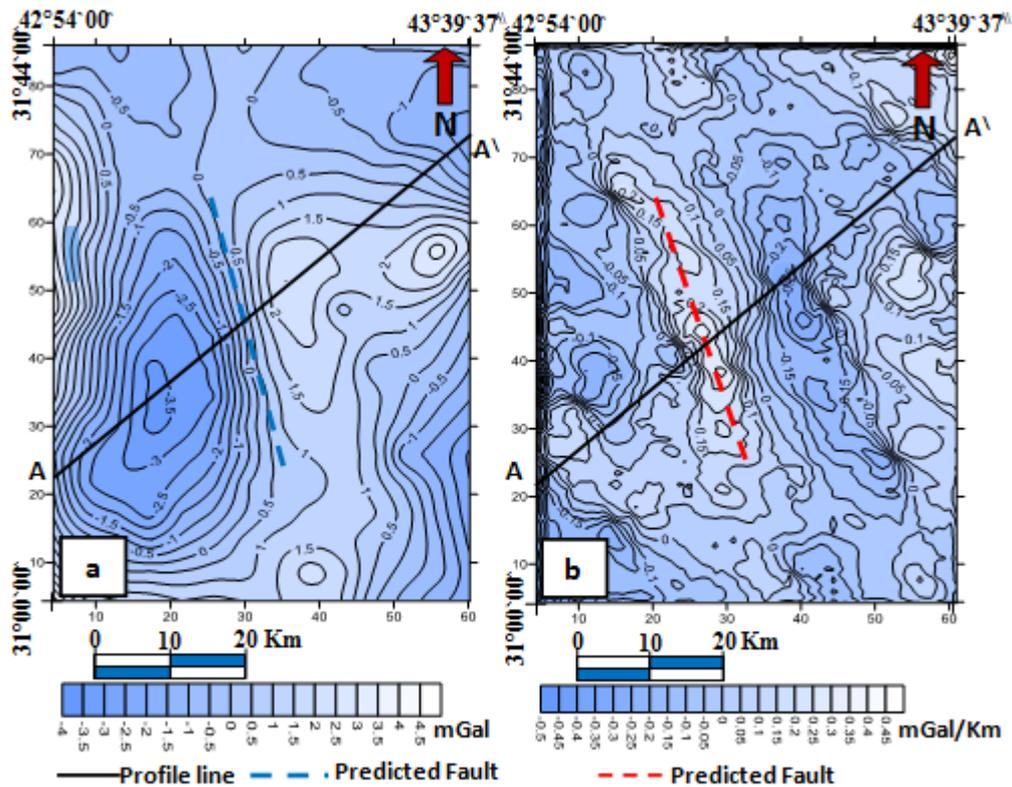
Figure 8- a) The residual gravity anomaly map showing the profile line A-A', and the predicted major fault line ; b) the horizontal gradient map.
