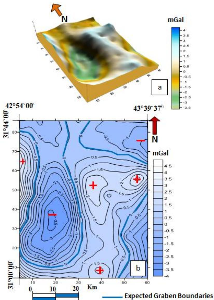
**Figure 5-** The Residual gravity anomaly: a) as a 3D- surface showing a typical graben structure; b) as a contour map showing the graben boundaries of zero value contour lines.
