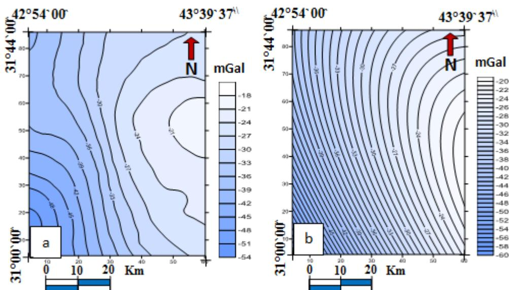
Figure 4- a) the total gravity anomaly field ; b) the regional gravity anomaly field
