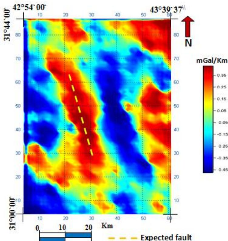
Figure 6- The horizontal gradient for the residual anomaly showing the probable faulting line over maximum values.
