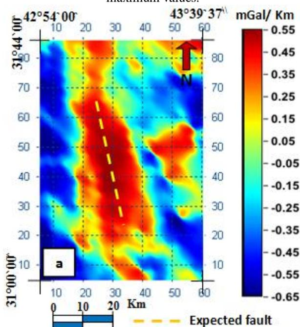
Figure 7- a) The 1<sup>st</sup> directional derivative for the residual gravity anomaly with the direction NE-SW showing the probable major fault line.
