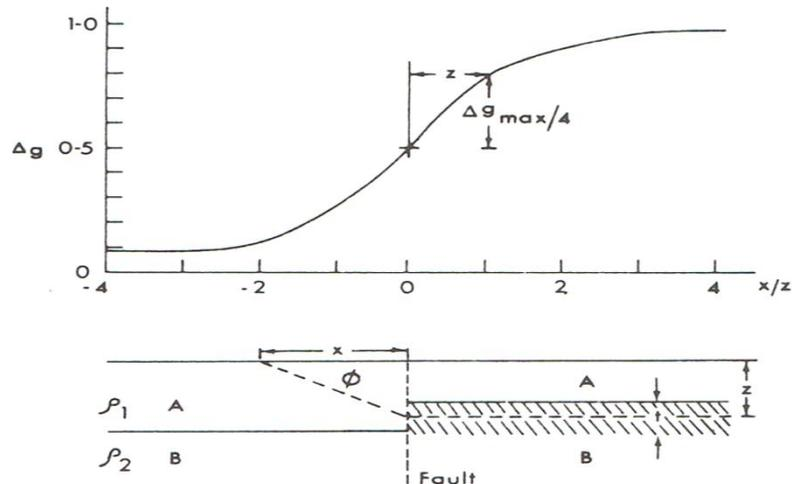
**Figure 10-** Gravity anomaly across a fault. Over fault trace the total change in gravity ( $\Delta g_{max}$ ) represents its half value. The horizontal distance over which the anomaly changes from  $0.5\Delta g_{max}$  to  $0.25\Delta g_{max}$  is a measure for the depth  $Z$ , after [1].
