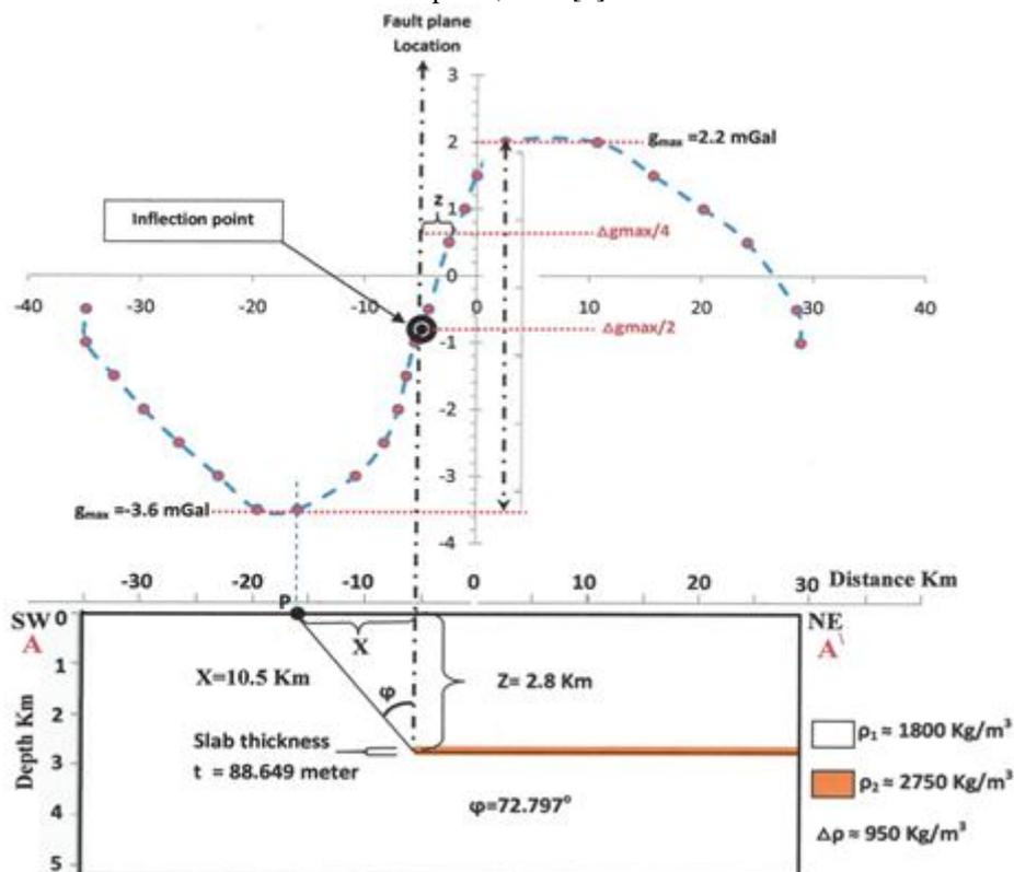
**Figure 11-** The geometrical model for the residual gravity anomaly along the profile (A-A') showing the quantitative interpretation of the expected major fault.
