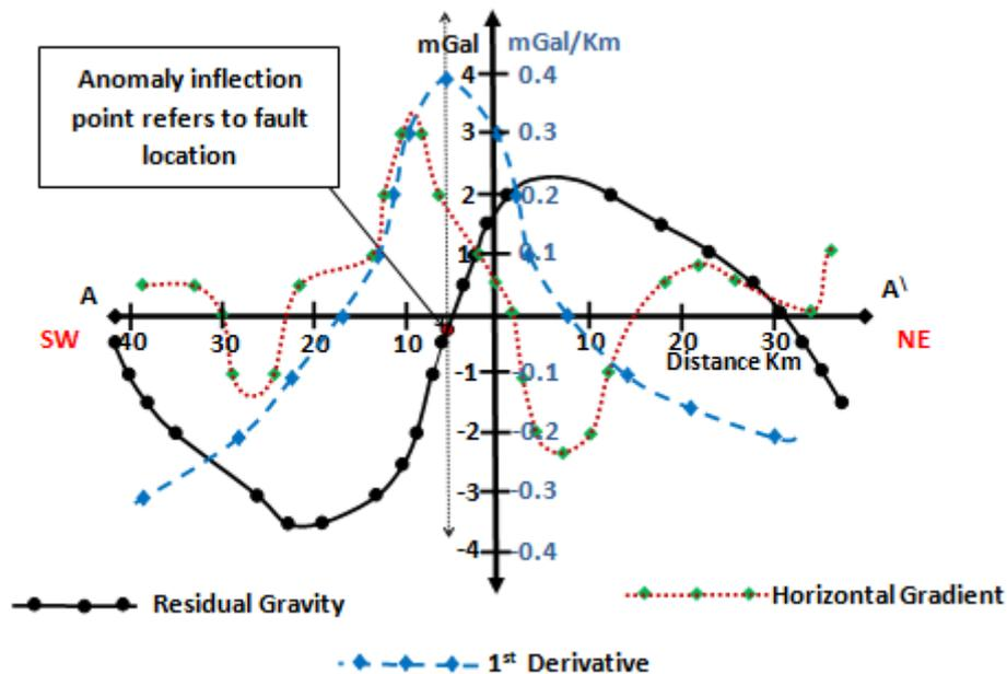
Figure 9- a comparison among the gravity residual field, 1<sup>st</sup> derivative and horizontal gradient along the profile A-A', showing the expected location of the major fault.
