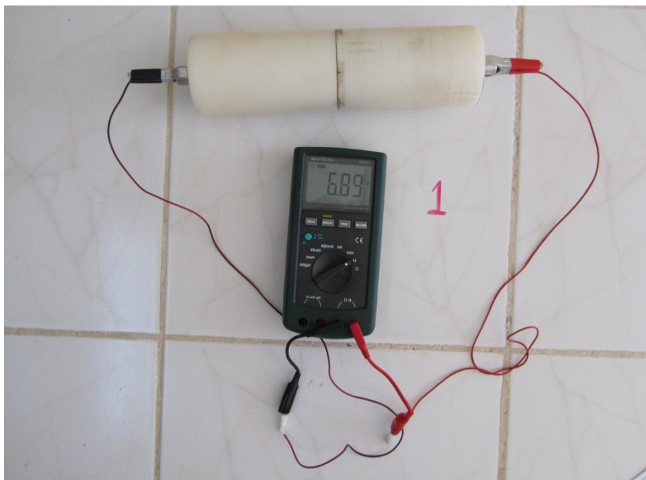
Figure 5- Shows circular metallic plate electrodes plugs directly into the Live terminals of the LCR meter.
