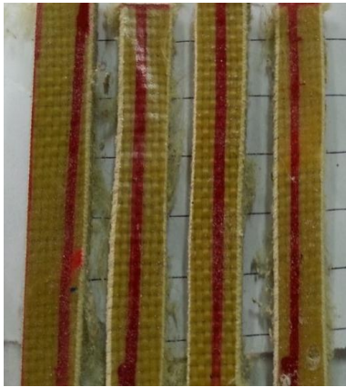
Figure 3- Samples of Impact Strength for (EP(80%)+UPE(20%)+K)
