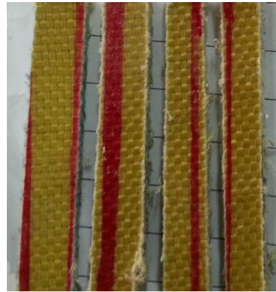
Figure 4- Samples of Impact Strength for (EP(80%)+UPE(20%)+K+Fe)
