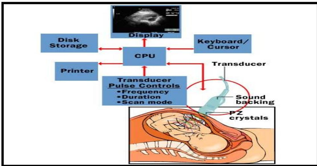
**Figure1-**The parts of an ultrasound machine[internet web site-www.physics.utoronto.ca].
