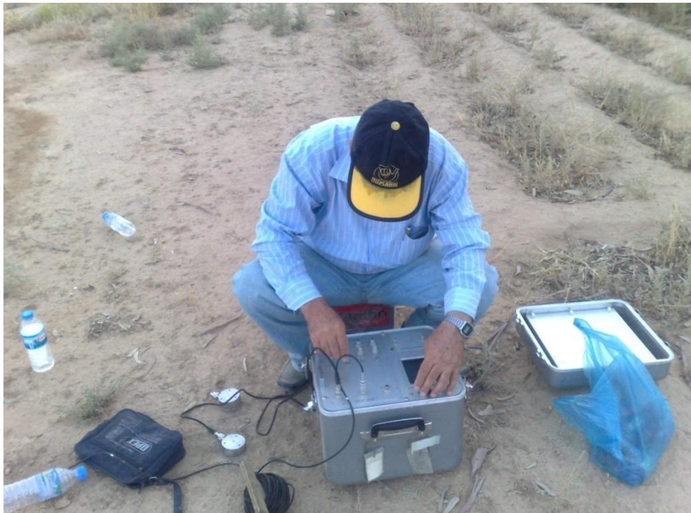
Plate 1- Field work at Al Jadiriyah area for measuring ( V_p ) and ( V_s ) velocities.
