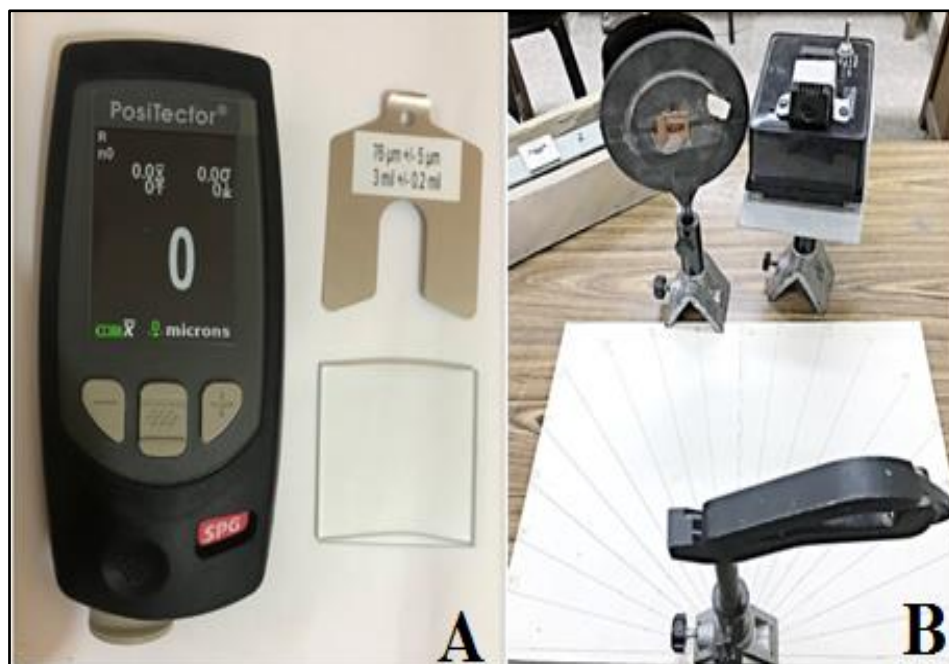
Figure 4- A) PosiTector device with a digital screen and probe type SPG used to measure the roughness of the magnetite surface; B) Laser Beam System used for measuring the reflectance (%) of the polished magnetite surface.
