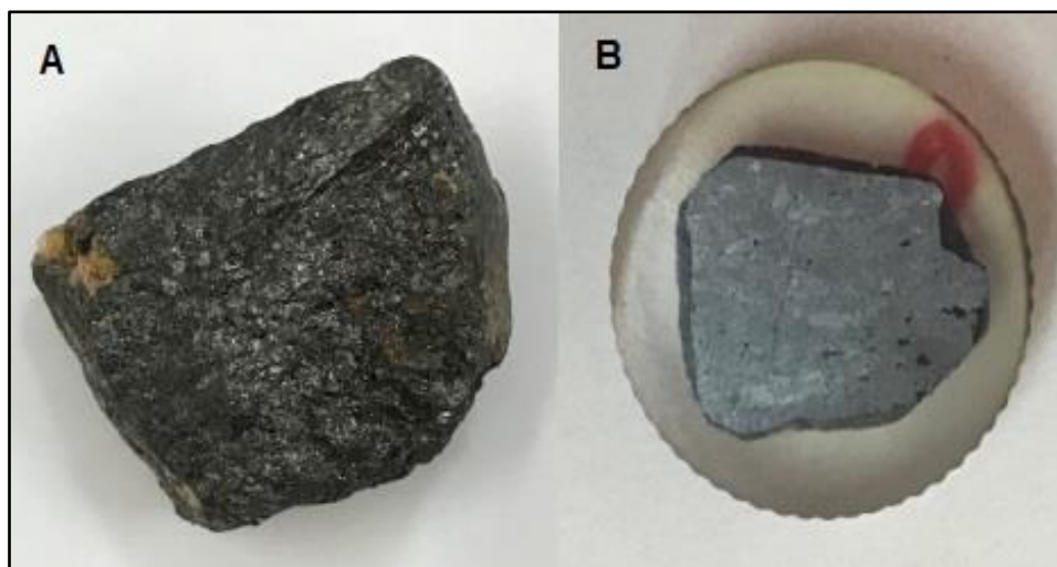
Figure 3- A Hand specimens of a magnetite displays a normal surface, B: section of magnetite used for testing the efficiency of the abrasive in polishing process.
