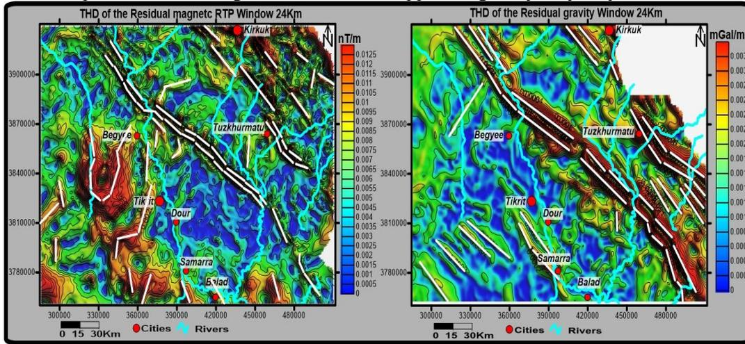
Figure 5- The total horizontal derivative (THD) of residual space windows 24Km of the gravity and magnetic data shows lineaments features.
