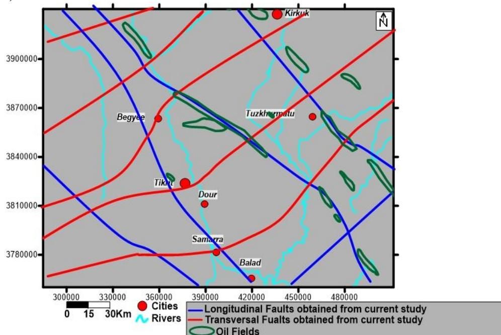
**Figure 9-** Basic tectonic boundaries lines estimated from gravity and magnetic lineaments.
