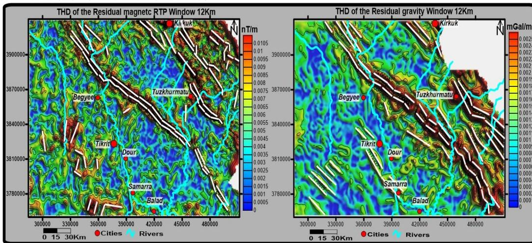
Figure 6- The total horizontal derivative (THD) of residual space windows 12Km of the gravity and magnetic data shows lineaments features.
