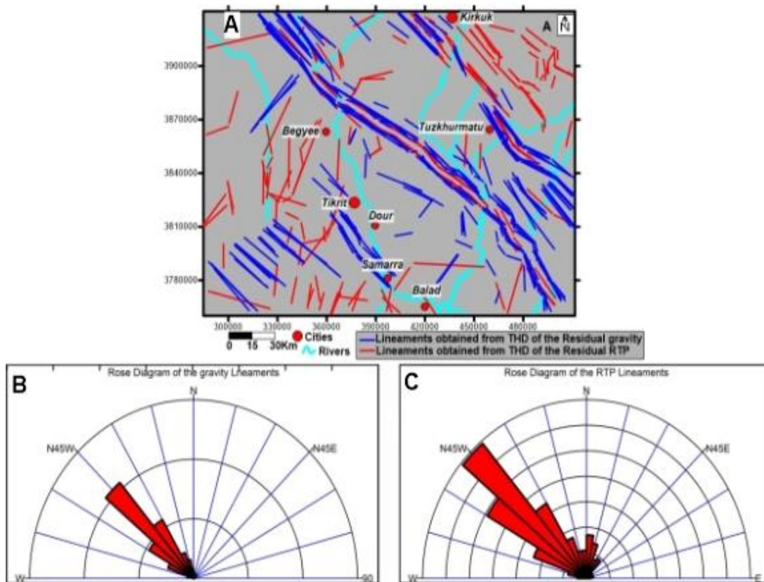
**Figure 8-** A- The lineaments features map for gravity and magnetic. B- Rose diagram for lineaments features from residual gravity data. C- Rose diagram for lineaments features from residual RTP magnetic data.
