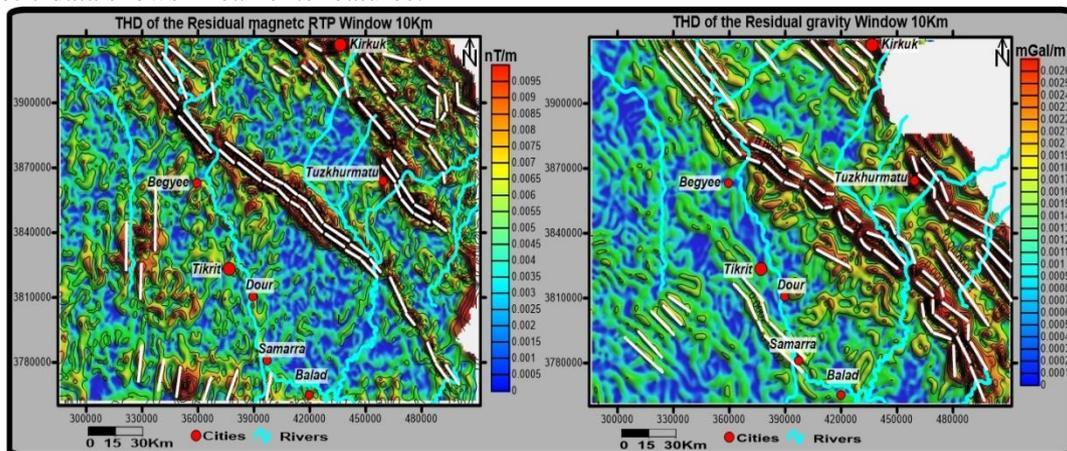
Figure 7- The total horizontal derivative (THD) of residual space windows 10Km of the gravity and magnetic data shows lineaments features.
