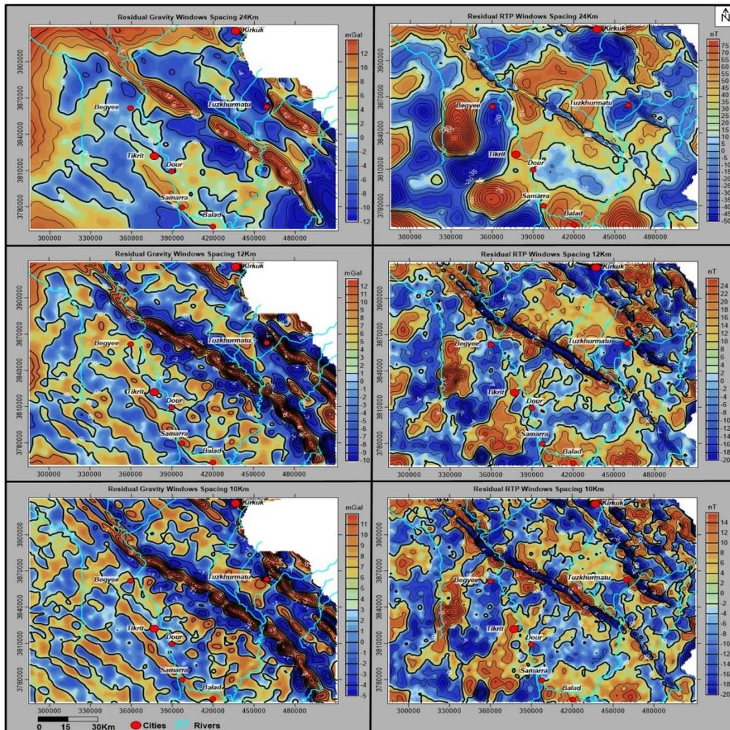
Figure 4- Residual gravity and magnetic maps of space windows 24, 12 and 10Km.
