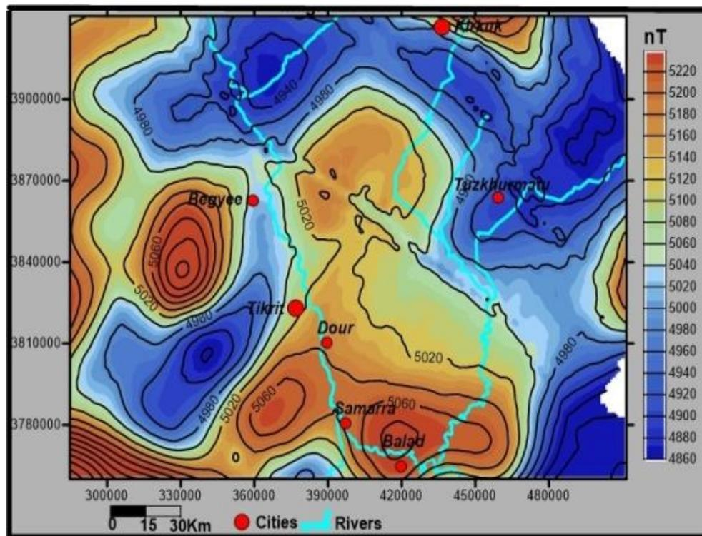
**Figure 3-** The Reduction to the pole (RTP) map of the study area.
