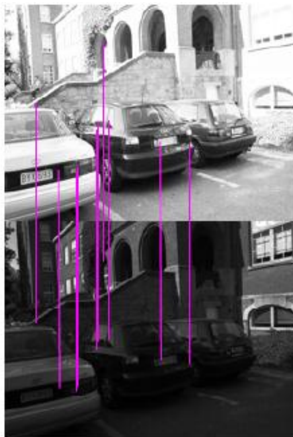
Figure 5- PCA-SIFT (shows the details of the first 10 matching keypoints between the darkest image and the brightest image using PCA-SIFT)
