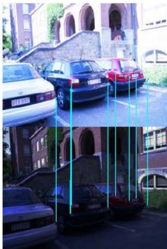
Figure 6-CSIFT (shows the details of the first 10 matching keypoints between the darkest image and the brightest image using CSIFT )
