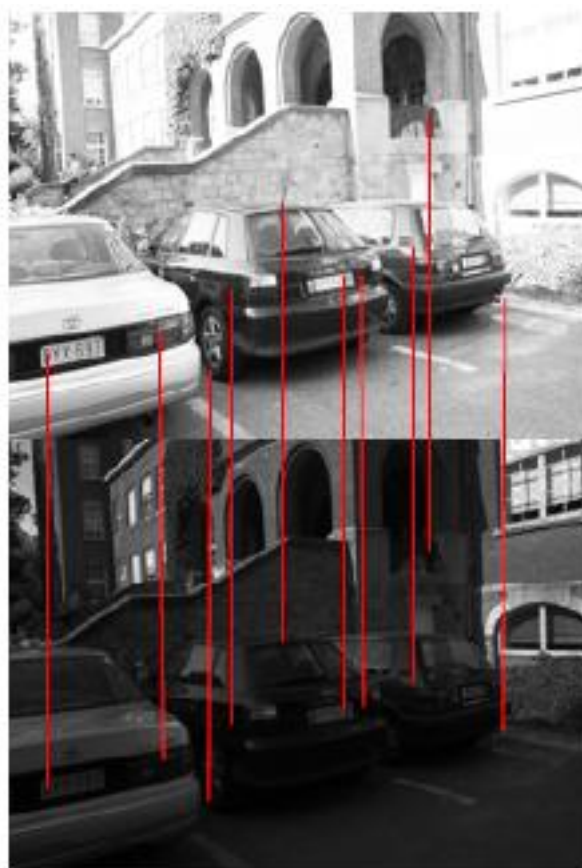
Figure 7- SURF (shows the details of the first 10 matching keypoints between the darkest image and the brightest image using SURF)
