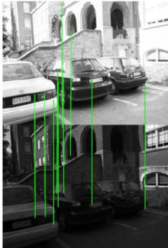
Figure 8- ASIFT (shows the details of the first 10 matching keypoints between the darkest image and the brightest image using ASIFT)
