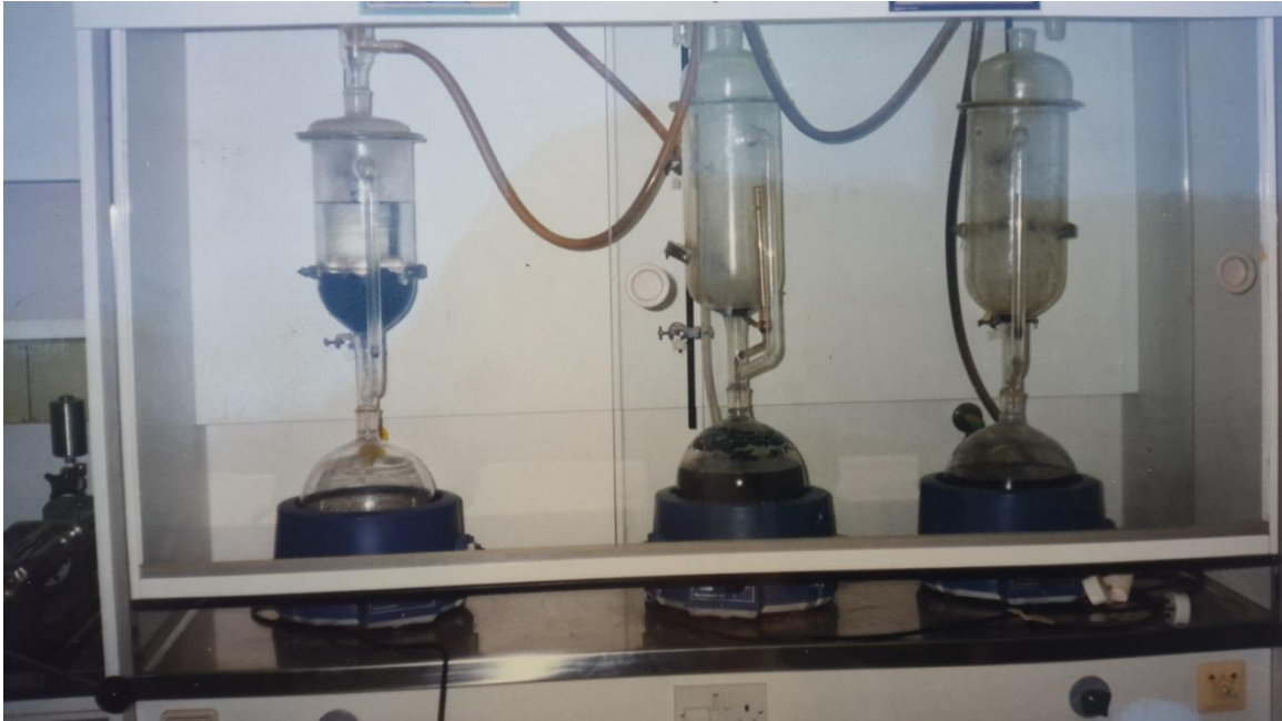
Plate 1- Shows the Soxhlet extractor instrument used for cleaning core samples.
