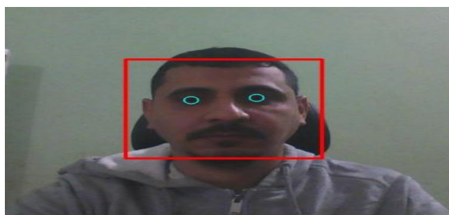
Figure 6- Haar-cascade detection in OpenCV.
