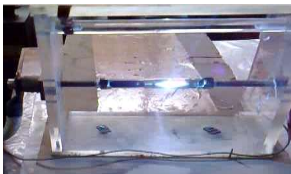
Figure 4- Cylindrically-tipped electrodes during a typical self-breakdown stage.
