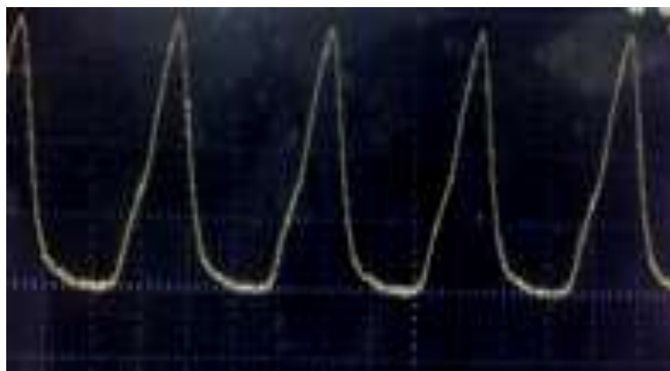
Figure 10- The output signal from PTh/f-MWCNT with load ratio 5wt% of CNTs photoconductive detector illuminated with IR radiation from diode laser of 808nm wavelength and incident power of 300 mW.
