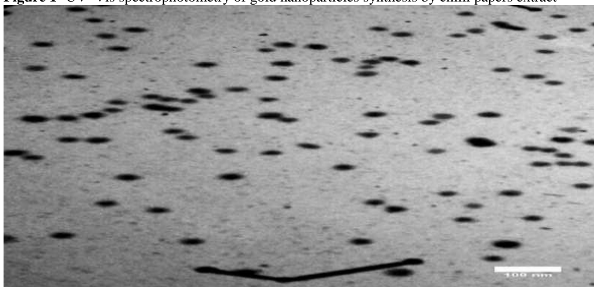
Figure 2- Transmission electron microscopic (TEM) images of Au NPs Synthesized using chilli papers extract.
