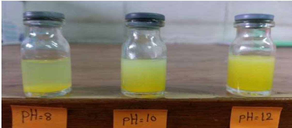
Figure 4- A photograph plate for samples of CdS QDs with different pH values (8, 10 and 12).
