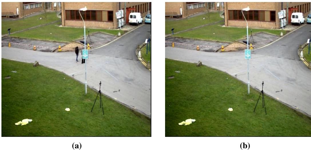
Figure 1- initial background (a): buffer using first 100 frame, (b): buffer using proposed method
