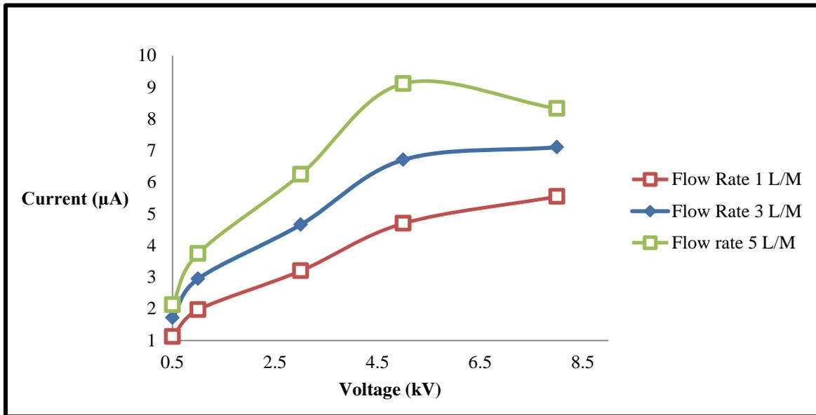
**Figure 4**-shows the relationship between the current as a function of the voltages and a different flow of argon gas (1, 3, 5  $l/min$ ).
