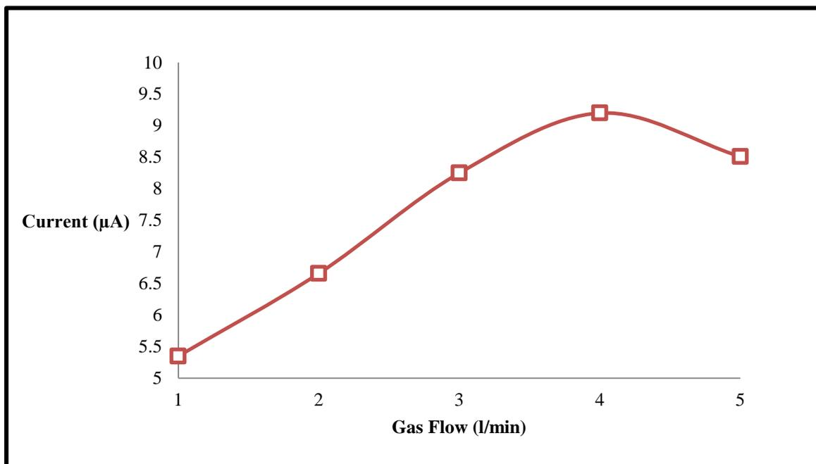
**Figure 6**-shows the relationship between the current as a function of the flow of gas at a voltage of (8)kV.
