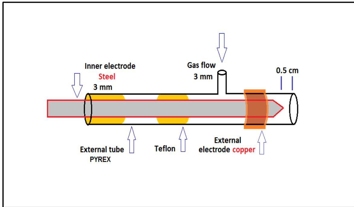
**Figure-1** Schematic for design non thermal plasma needle.
