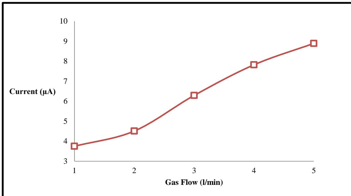
**Figure 5**-shows the relationship between the current as a function of the flow of gas at a voltage of (4.9)kV.
