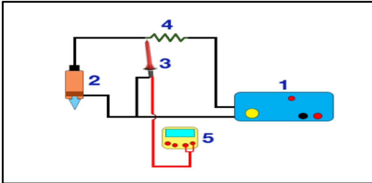
**Figure 3-**Schema illustrating connection of an electrical circuit of non-thermal plasma needle system, where: 1- HV power supply, 2- non-thermal plasma needle, 3- HV probe, 4- resistor 8  $\Omega$ , 5- Digital multimeter.
