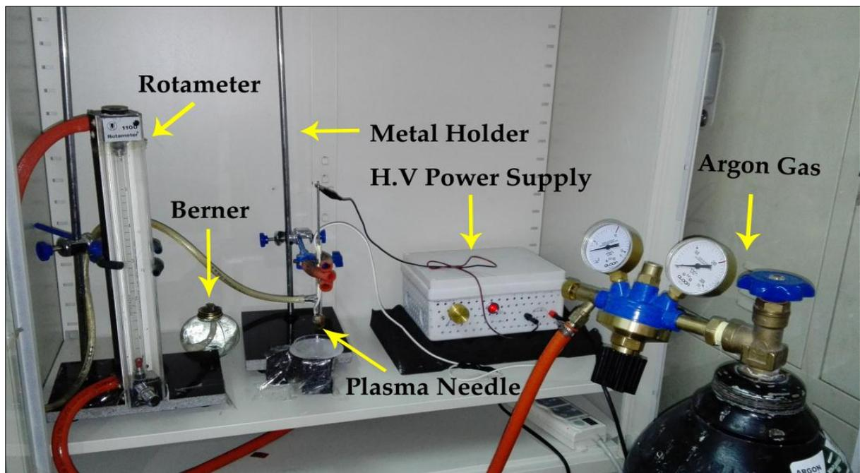
**Figure 2-**Image of Non-Thermal Plasma Needle System.
