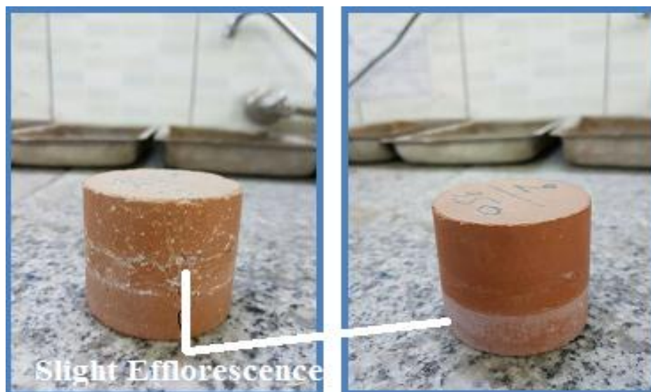
Figure7- Efflorescence process of brick samples prepared by pressing the two sites (DH2, S) and burned at 950 C°.
