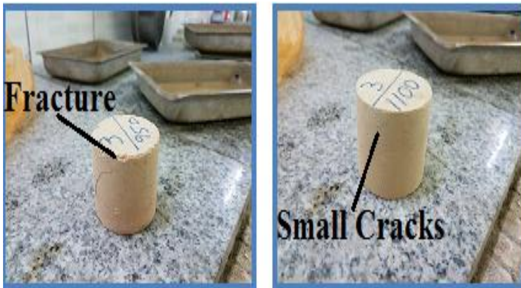
Figure6- The outer shape of the brick samples prepared by pressing the third position (S)
