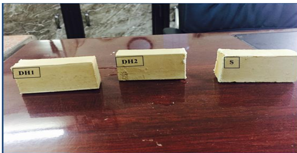
Figure 4- The colors of the samples of the blocks prepared by extruding and burned at a temperature (950) C°.
