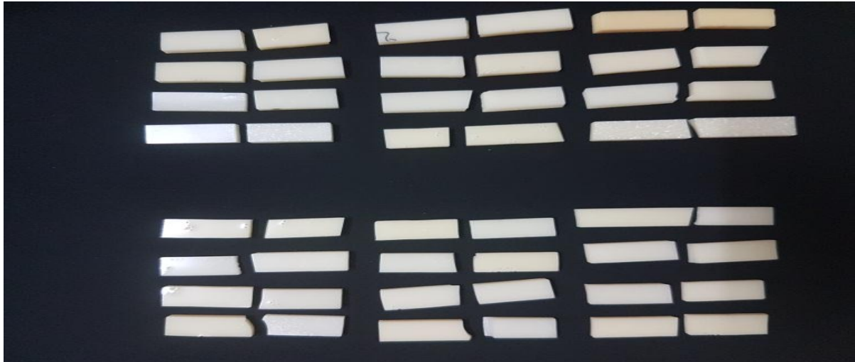
Figure 2- The impact strength specimens that were tested before and during immersion in water for 10 weeks.
