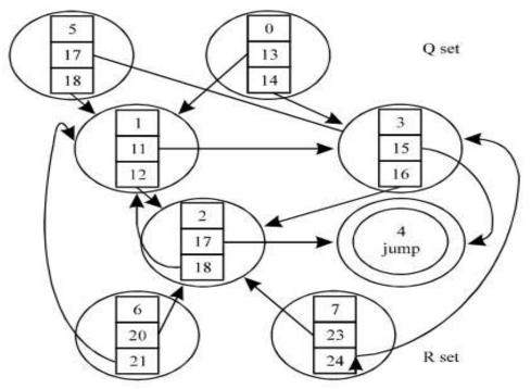
Figure 2-Transition Design of RADG [8].
